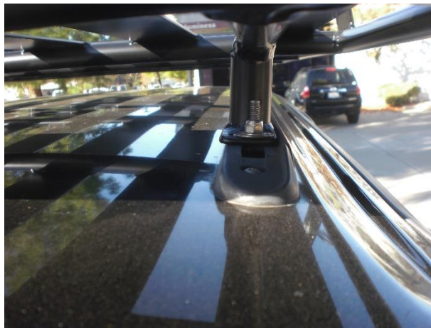
Figure 1: Roof Rack Mounted into Place
