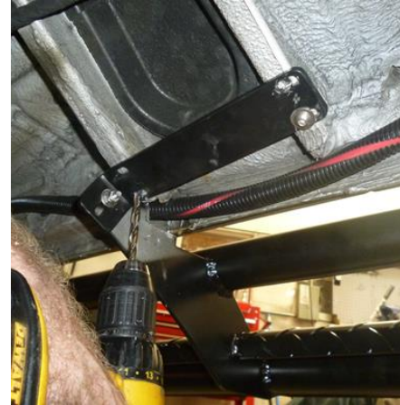
Figure 7: Center Mounting Bracket Against Front Body Brace.
