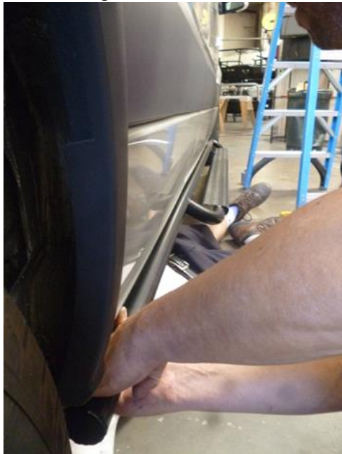
Figure 6: Pull Nerf Bar to Align with Van Contour.
