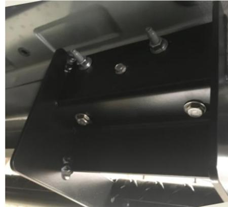
Figure 3: Hardware Installed Through Nerf Bar Brackets
