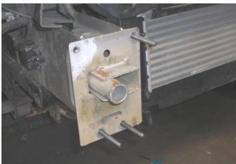
Figure 13: Frame Profile After Cutting
