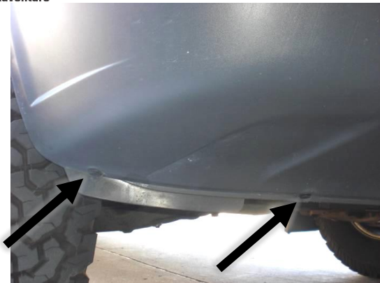
Figure 6: Plastic Fastener Locations Under Leading Edge of Bumper
