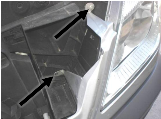
Figure 7: Headlight Trim Piece Torx Bolts
