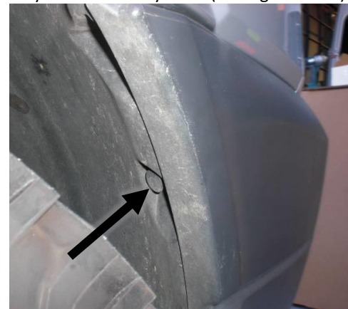
Figure 5: Plastic Fastener Location in Fender Well
