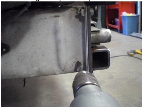
Figure 17: Drill Two (2) Equally Spaced 7/16" Holes Through the Frame (One (1) Hole Through Frame per Side)
