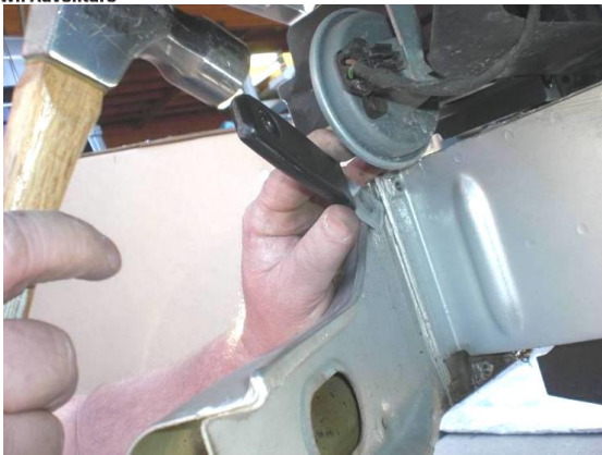
Figure 11: Releasing Stock Bumper with Hammer and Putty Knife
