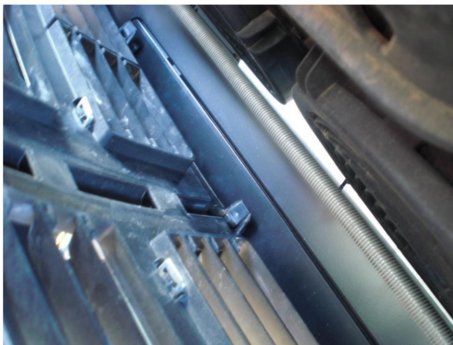
Figure 13: Stock grill installed on Aluminess door tabs
