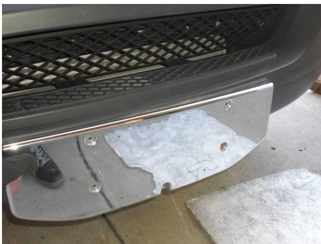
Plate cover (left) and plate cover removed (right) showing bumper cover fasteners
