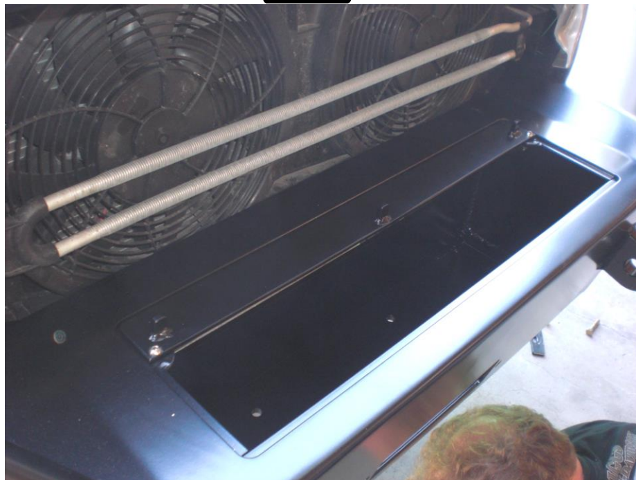
Figure 12: Bumper door, rear portion installed
