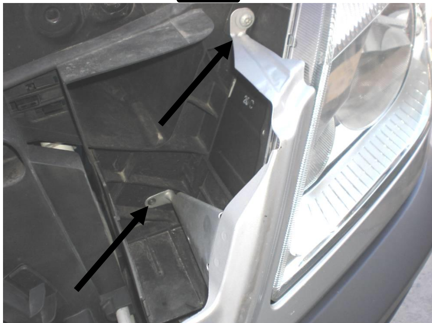
Figure 5: Headlight trim piece torx bolts
