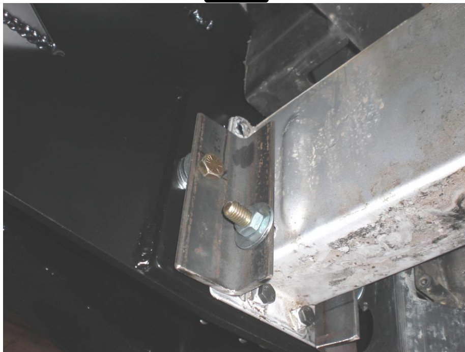
Figure 11: Steel support brackets bolted to frame
