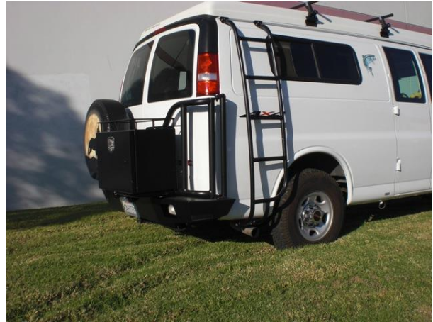
Figure 1. Passenger Side Ladder Installed
