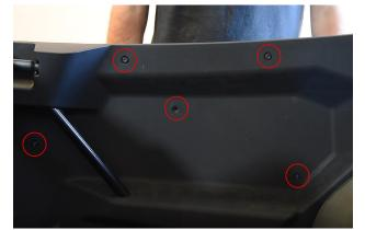
1. Remove the stock bolts from the door (shown in picture).
