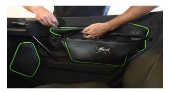
Then in the upper-front bolt hole inside the bag, install the supplied (1x) 1.25" Phillips Head (Larger) with (1x) <sup>1</sup>/<sub>4</sub>" Washers.
