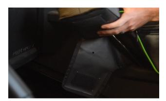
7. For the Knee pad section, seperate the pad from the Ktex backing (Pull apart the Velcro). Line up the guide hole in the Ktex with the bolt hole in the door. Then install the supplied (1x) 1.25" Phillips Head (Larger) with (1x) 1/4" Washers.
