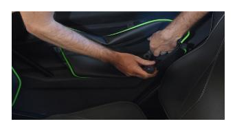
4. Unzip the door bag, and line up the two guide holes inside the back of the bag with the corresponding bolt locations on the door.
