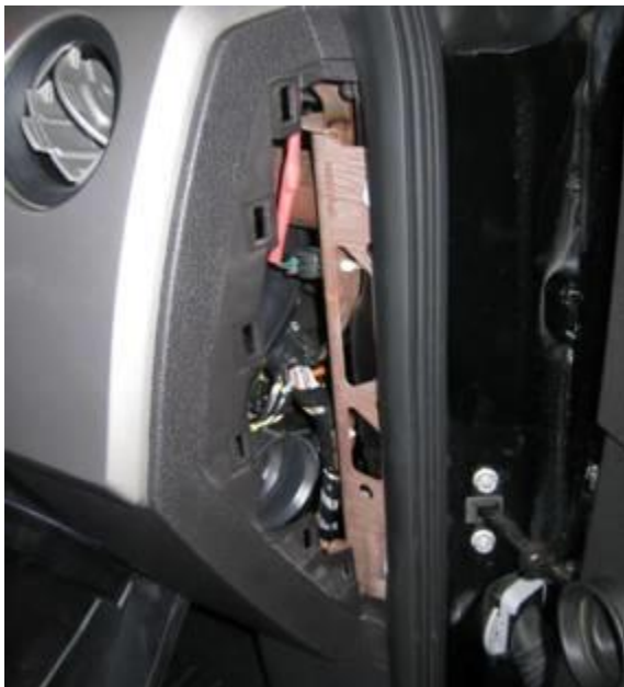
View of side panel removed to allow removal of glove box.
