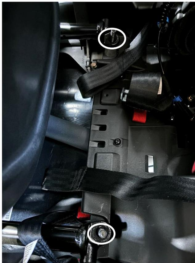
**Step 5:** Use 5/8" socket to remove the seat belt strap mounting bolt on the right side of the driver seat.
