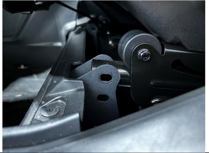
**Step 4:** Using a 18mm socket, remove the nuts on the rear of the seat.
