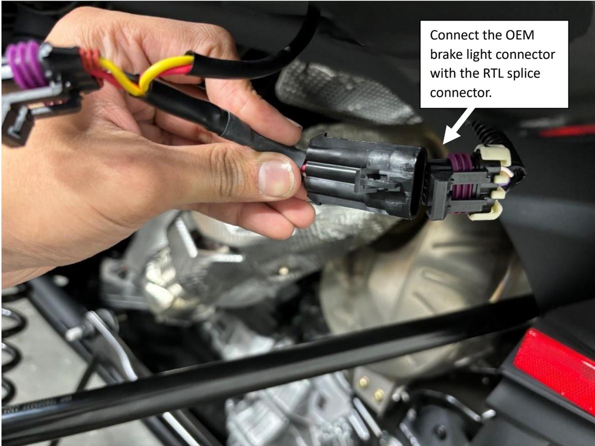
Connect the splice adapter with the brake light connector on the vehicle.
