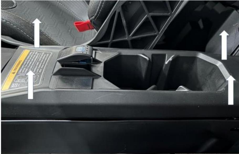
**Step 16:** Carefully pull out the switch panel on the lower console. This will create an empty space that would be used to pull the spade connectors for mounting the switches.
