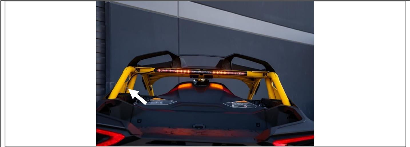
**Step 10:** Follow the route shown in the photo to run the connector near the Brake light.
