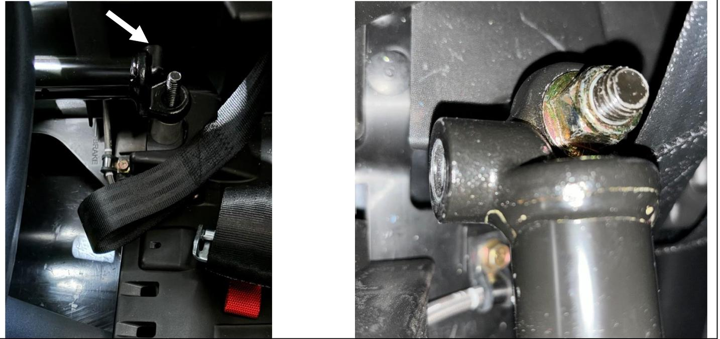
**Step 6:** Carefully remove the seat belts and seat.
