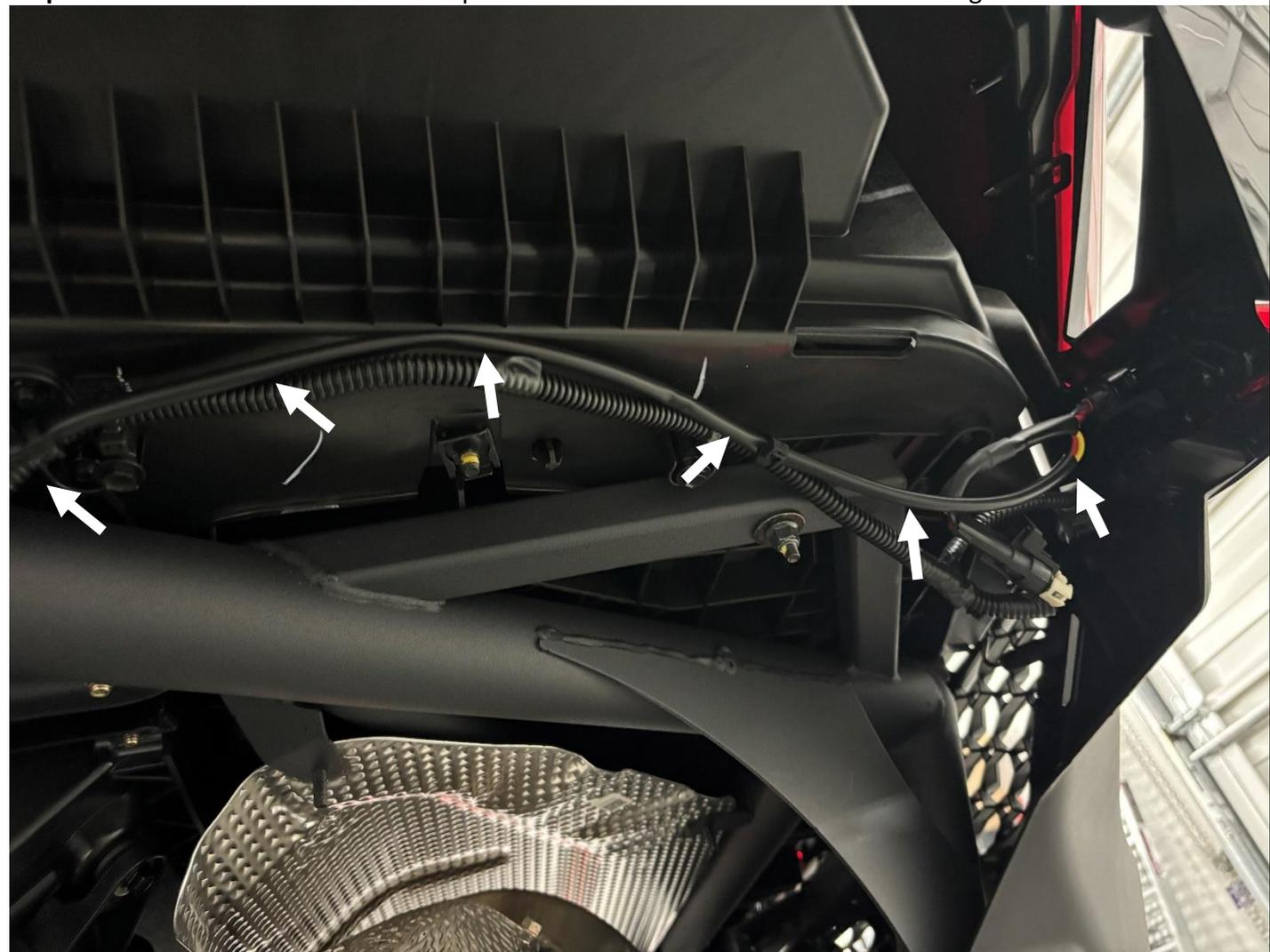
**Step 11:** Connect the harness bullet connectors with the RTL splice adapter by matching color to color as shown in the photo.
