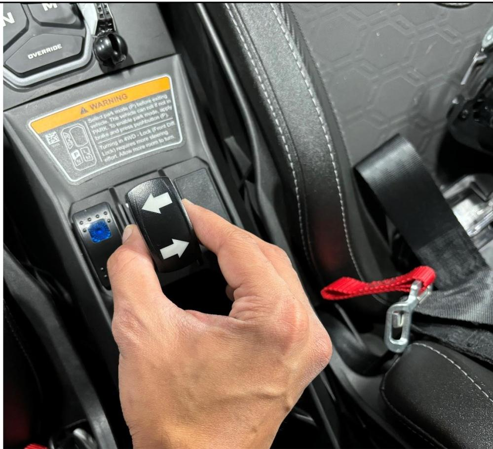
**Step 18b:** For the reverse switch, drill a  $\frac{3}{4}$ " hole in the punchout as shown in the photo.
