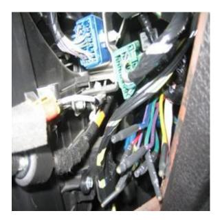
The other 4 wires behind the glove box are the "pass through" harness that Ford installed from the factory to pass through the firewall and end above the passenger side wheel well in the engine bay.
