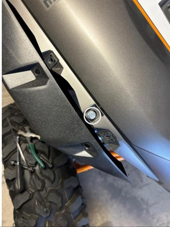
**Step 6: Remove metal clip underneath the fender flare**
