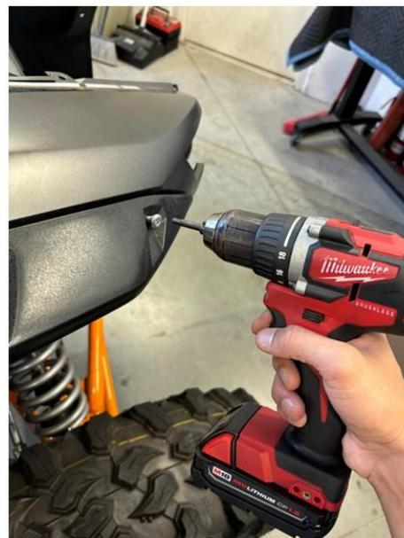
**Step 5: Remove flange bolt under the fender flare.**
