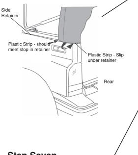
**Step Seven** SECURE TENSION STRAP
