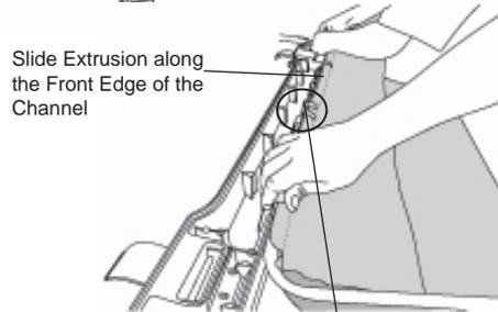
Line up the Center Notch in the Fabric with the Center Notch in the Header
