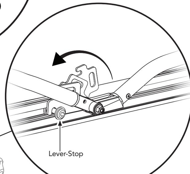
Engage the Locking Lever on both sides of the truck.
