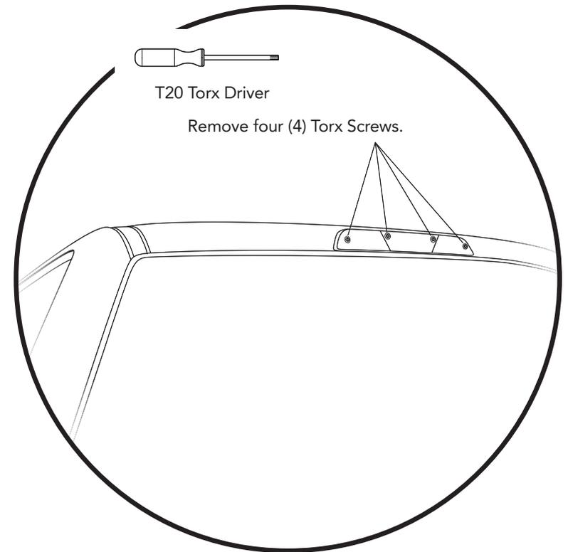
Use a T20 Torx Driver to remove the 4 screws that attach the Center High-Mounted Stop Light to the vehicle cab, and remove the CHMSL.
