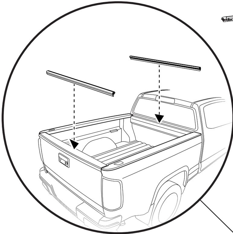
Place the Front Rail and Rear Rail onto the truck bed.
