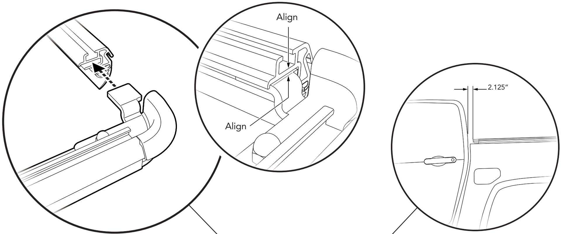
Attach the Front and Rear Rails to the Side Rail Assemblies.
