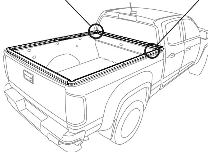
Place the outer edge of both side rail corners 2.125" from the back side of the vehicle cab.
