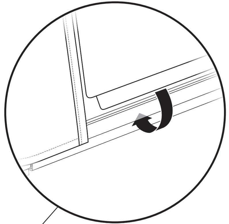
Tuck the plastic tab along the bottom edge of each Side Curtain into the slot along the side of each Side Rail.
