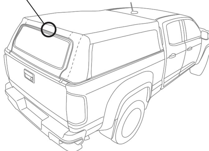
Feed the connector end of the CHMSL wire harness through the slit in the top fabric, and pull the wire all the way through both layers of fabric.
