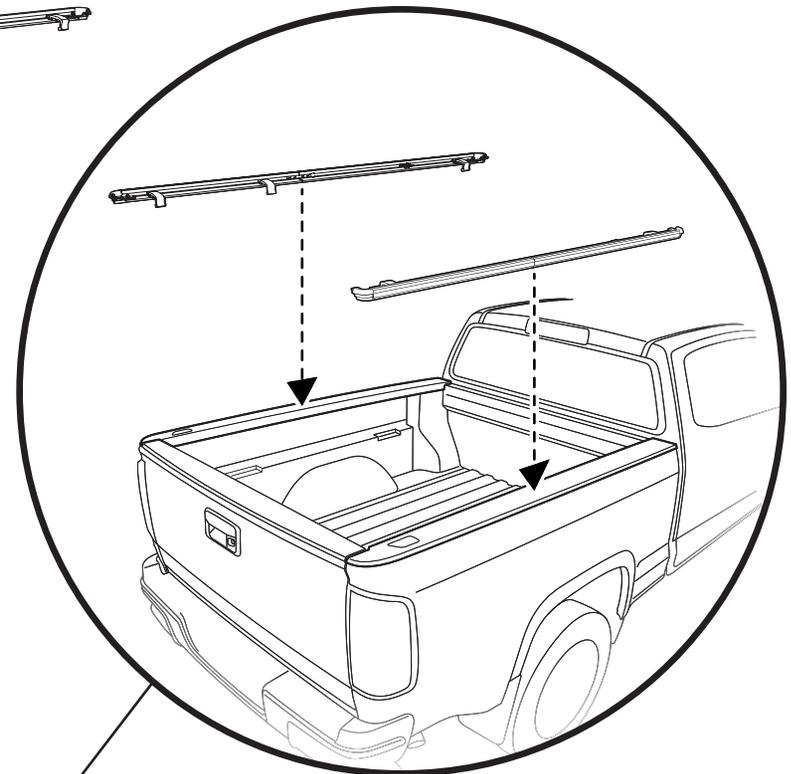
Place Side Rail assemblies onto the truck bed. Lay the Rails on top of the plastic bed protectors.
