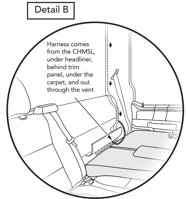
Route the 29' Wire Harness from the interior side of the CHMSL, above the headliner, down the rear driver side pillar, under the carpet, through the cab vent, into the vehicle bed, and along the top of the bed, underneath the bed rail cap. See Detail B.
