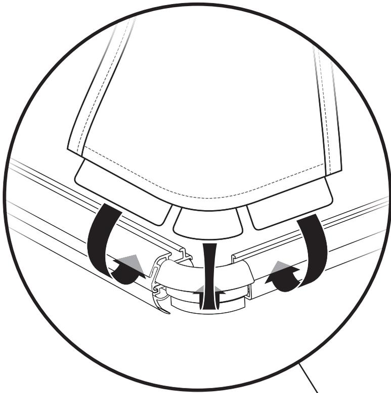
Tuck the plastic tabs at the bottom of each corner of the top into the slots in the Side Rails and Front and Rear Rails.
