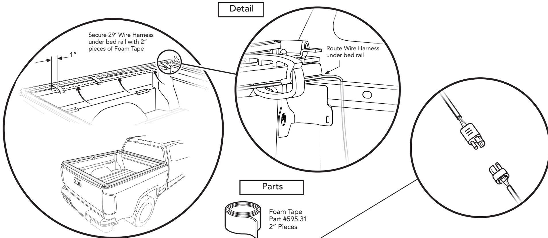
Route the 29' Wire Harness from the front of the vehicle bed to the rear, underneath the bed rail, and through each of the three clamps. (See Detail) Attach the wire to the underside of the bed rail using 2" pieces of the Foam Tape. Run the wire to just 1" past the rear clamp.
