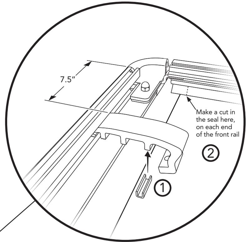
① Attach a Clamp Pad to each Upper Clamp on the Front Side Rails, on the rib farthest from the side rail.
