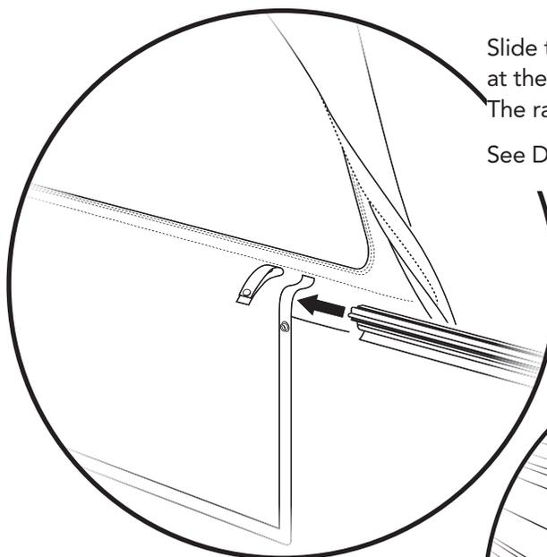
Slide the front rail onto the plastic retainer at the bottom of the front window. The rail should go under the large flap. See Detail.
