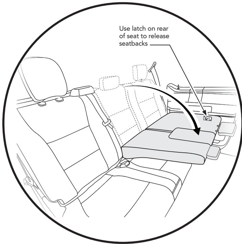
Use the latch on the rear of the driver side rear seatback to release the driver side and middle seatbacks, and flip both seatbacks forward.
