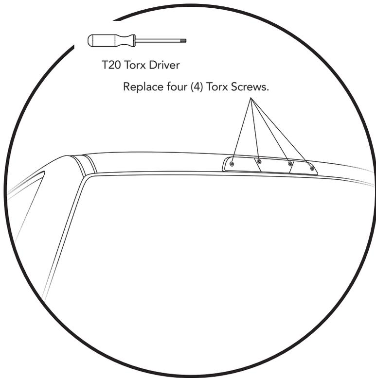
Find the four (4) T20 Torx screws you removed earlier, and re-attach the Center High-Mounted Stop Light (CHMSL) to the vehicle cab.
