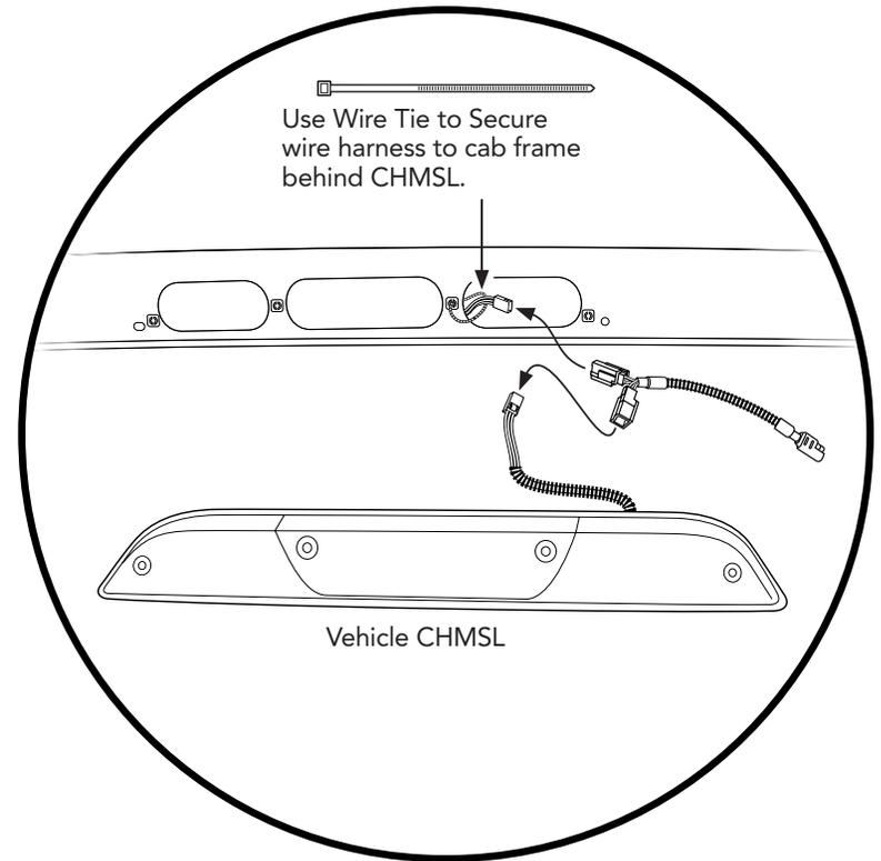
Use Wire Tie to Secure wire harness to cab frame behind CHMSL.
