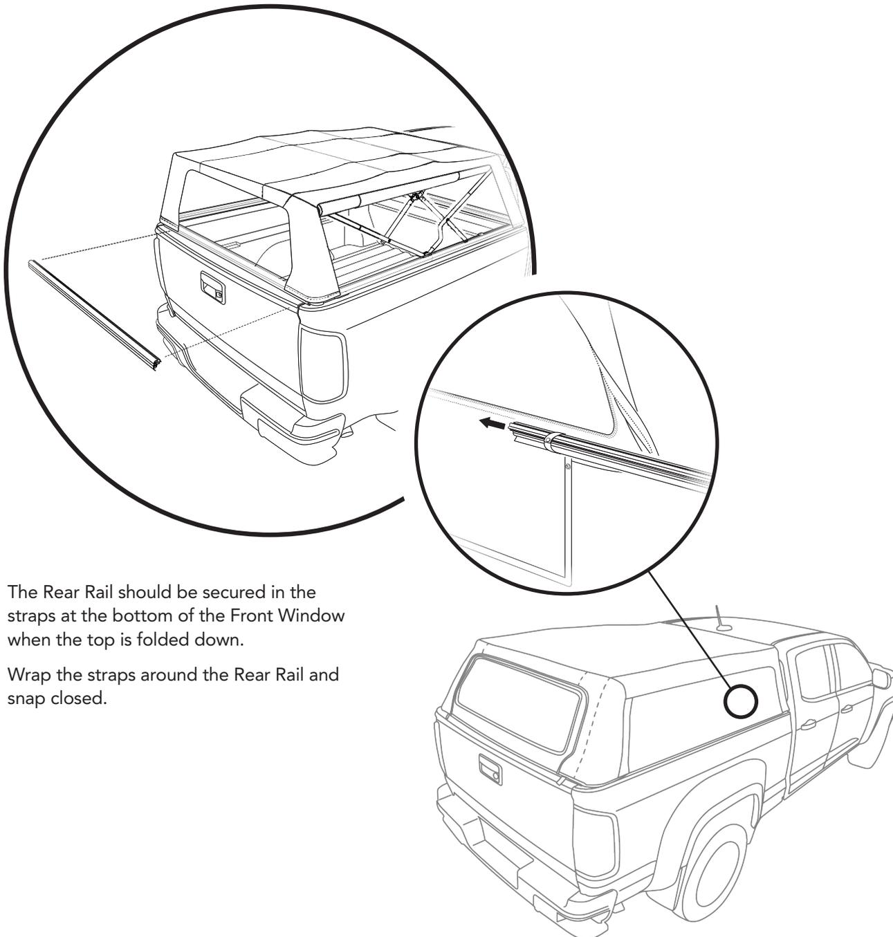
The Rear Rail should be secured in the straps at the bottom of the Front Window when the top is folded down.
