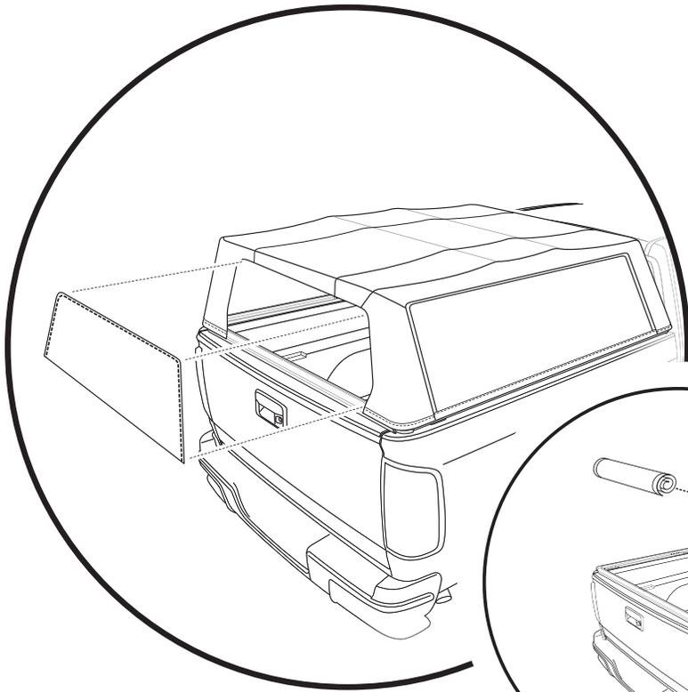
With the Fabric Top up, the Rear Window can be stored in the Boot attached to the bottom of the Front Window.
