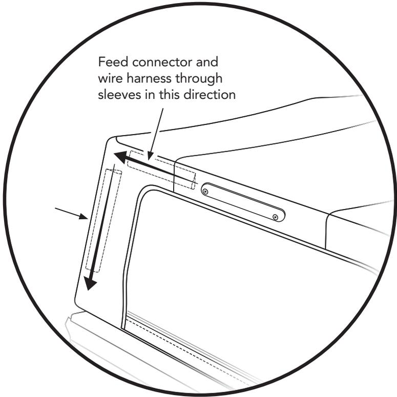
Feed the connector and wire harness through the fabric sleeves on the inside of the top.
