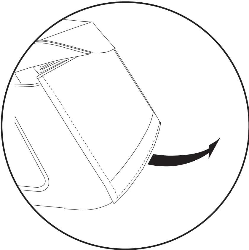
Open the Tailgate then pull back on the Tailgate Bar.
