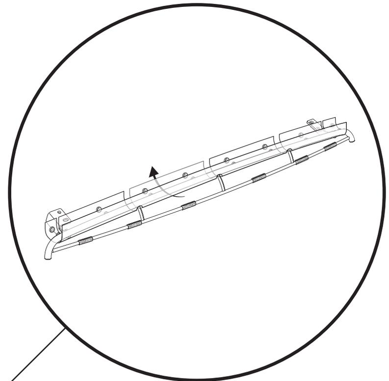
Flip the rear of the fabric deck forward for easier access.
