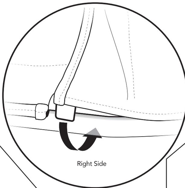
Tuck the plastic tabs at the bottom corners of the Rear Window under the Jeep belt rail.
