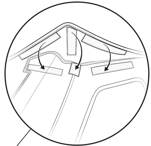
Locate the Hook & Loop strips at the rear corners of the top fabric.
