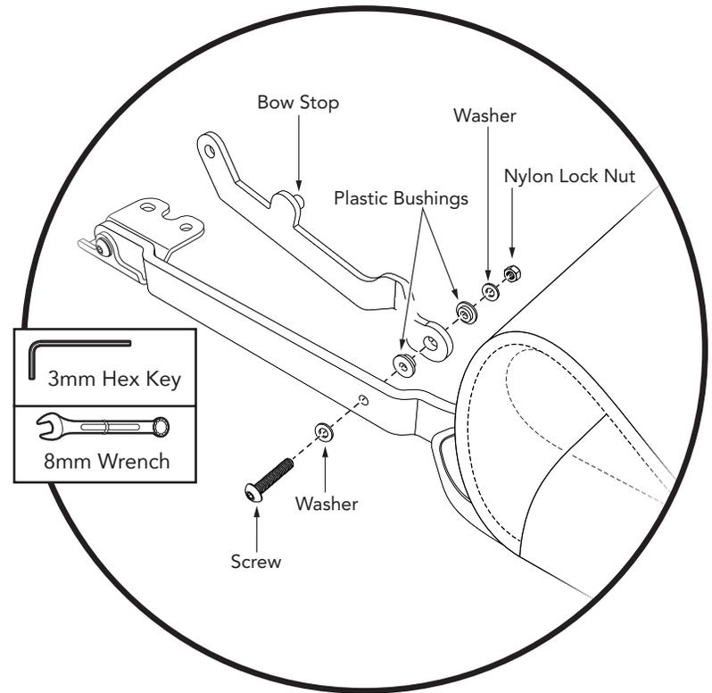
Attach the #2 Bow Link Assemblies to the Side Bows on the Header Assembly. Make sure that the Bow Stop on each Bow Link Assembly faces in.
