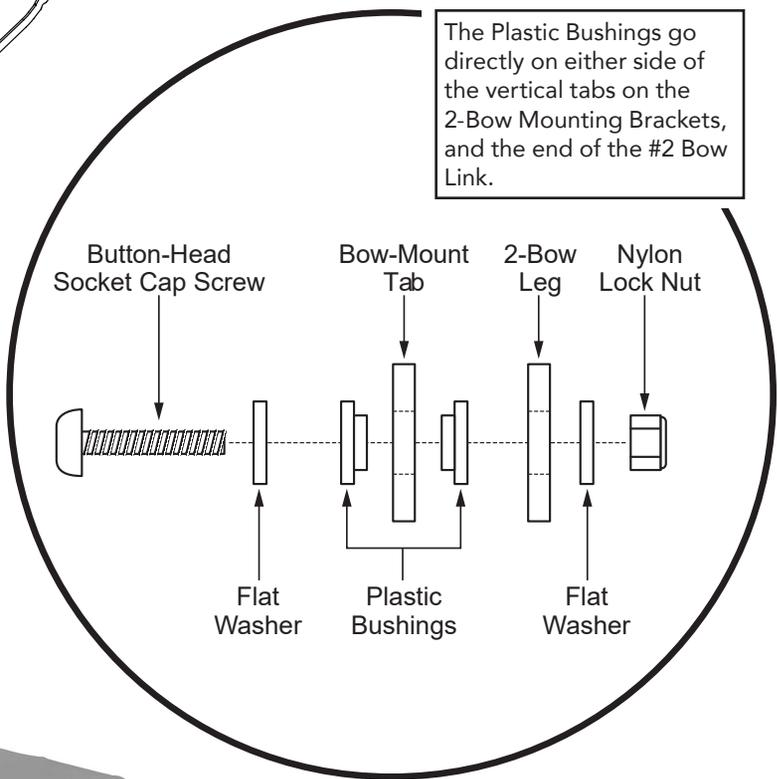
The Plastic Bushings go directly on either side of the vertical tabs on the 2-Bow Mounting Brackets, and the end of the #2 Bow Link.
