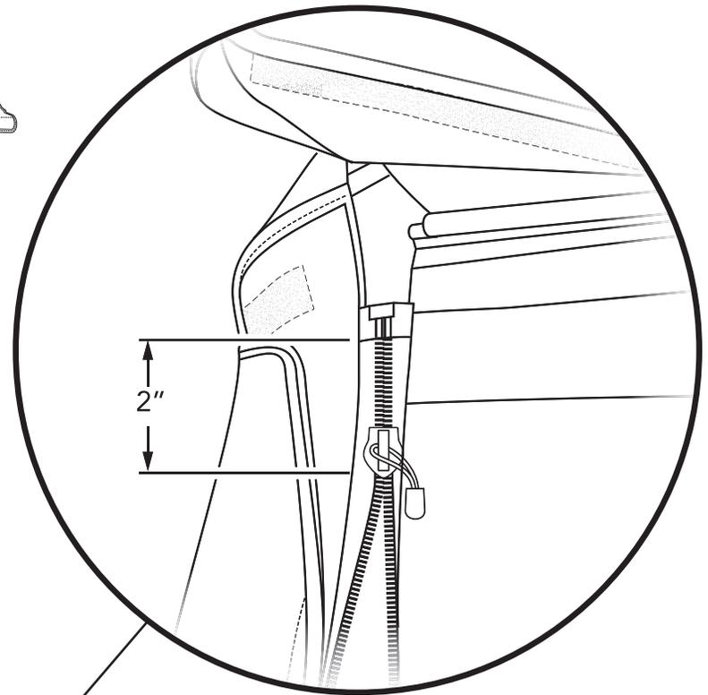
Lift up the corners of the Top Fabric to expose the Rear Window attachment channel.
