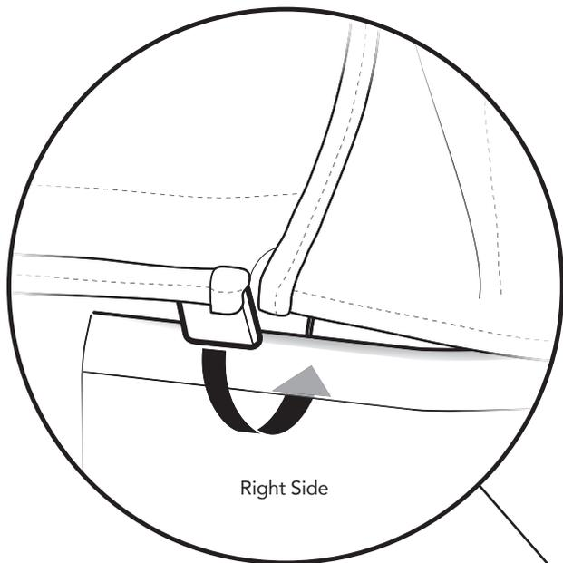
Tuck the plastic tab at the bottom rear corner of each Quarter Window under the Jeep belt rail.
