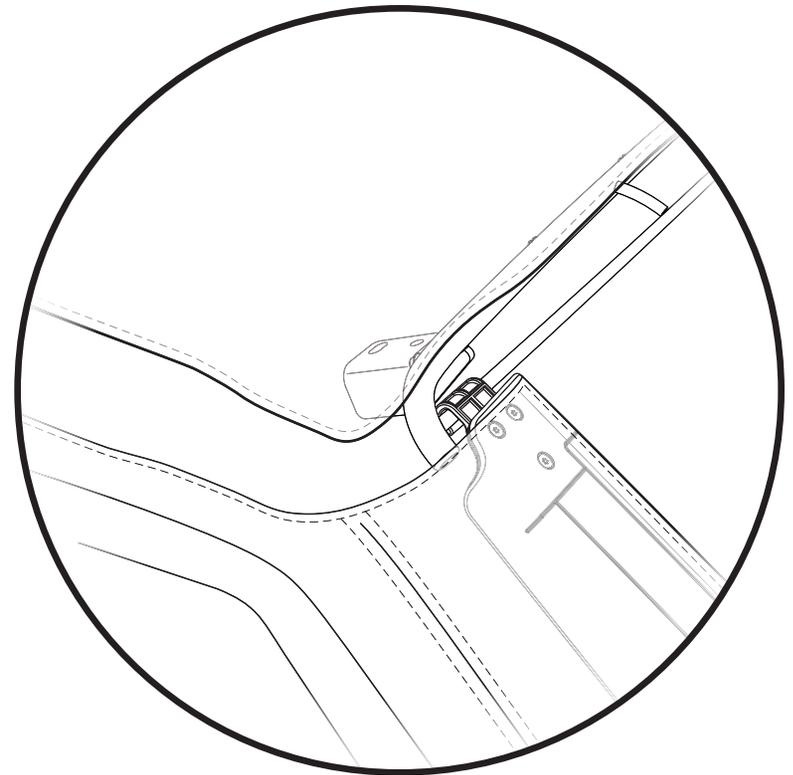
Attach the Quarter Window Stiffeners (attached to the inside of each Quarter Window) to the #4 Bow cross bar.
