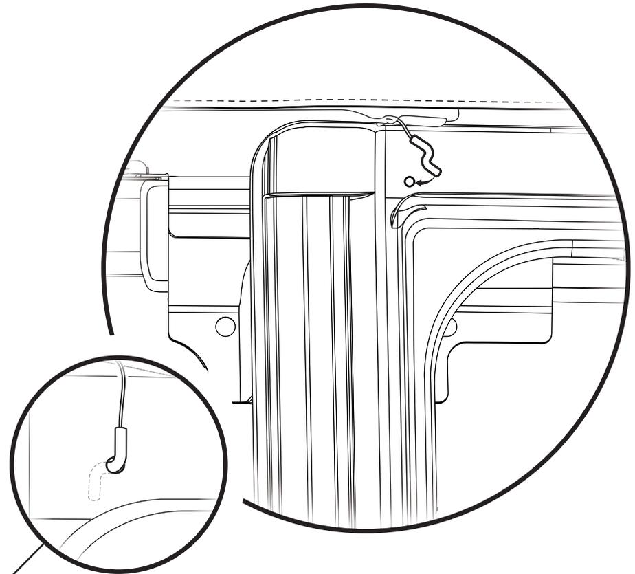
Locate the Z-Clips, which extend out from the edge of the top fabric just above the Door Rail on each side of the Jeep.
