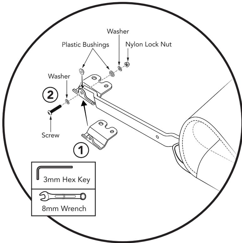
Attach the Side Bow Pivot Brackets to the Side Bows on the Header/Deck Assembly.
