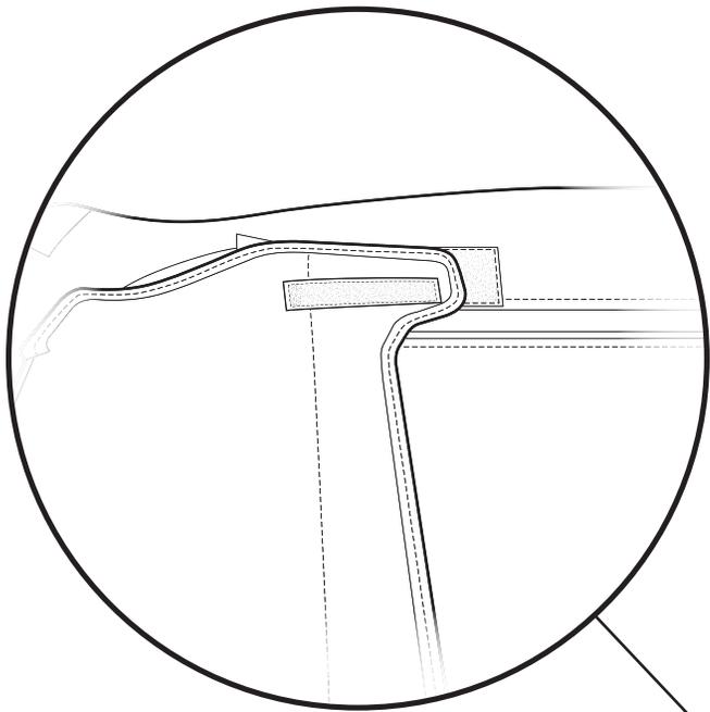
Locate the hook and loop strip at the left rear corner of the top fabric.
