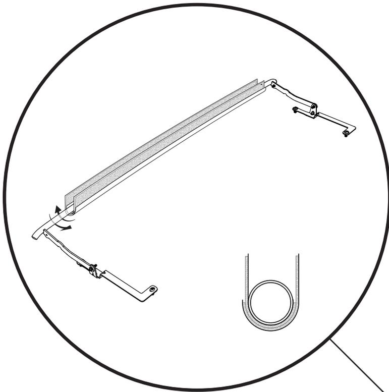
Locate the two fabric flaps sewn to the inside of the fabric top just above the #2 Bow.
