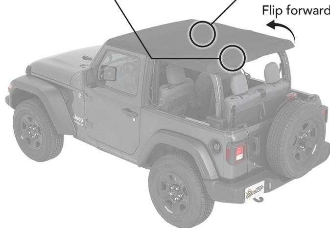
With the rear of the fabric deck flipped forward, locate the four flaps sewn to the inside of the fabric top just above the #4 Bow.
