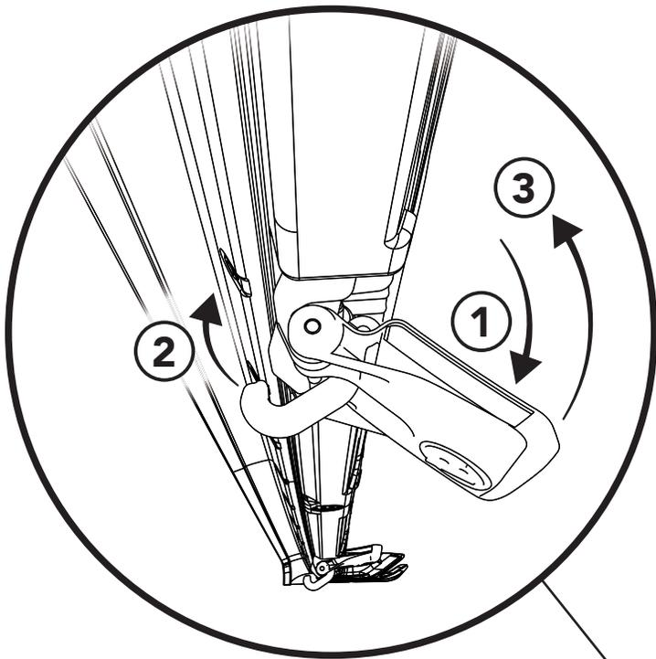
Fold the Sunrider closed and secure both latches to the vehicle's windshield header.
