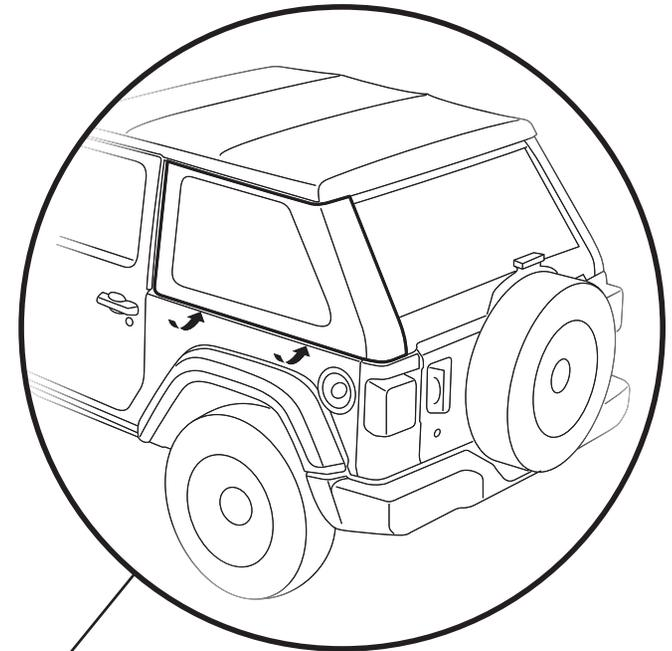
Locate the the sewn-in plastic strip along the front edge of the left Quarter Window.
