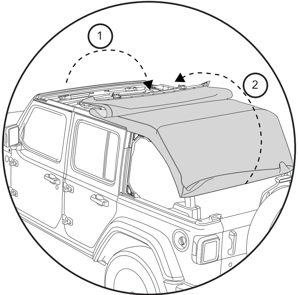
Lift the Top fabric assembly over the top of the vehicle.
