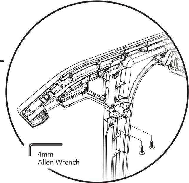
Attach the two (2) U-Clips to the Upper Rear Door Rails in the positions indicated. Make sure to have the threaded barrel of each U-Clip facing up.
