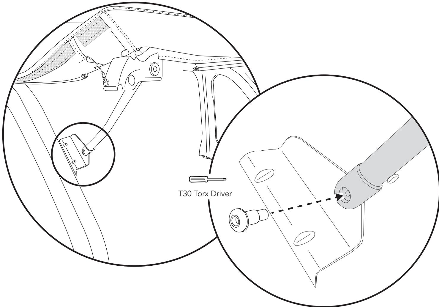
Attach the #6 Bow Support to the #6 Bow Mounting Brackets using one (1) Pivot Knuckle Screw per side.
