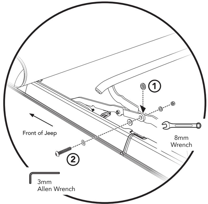
Attach the #Header/Deck/Side Bow Assembly to the top of the Front Door Rail rear brackets.
