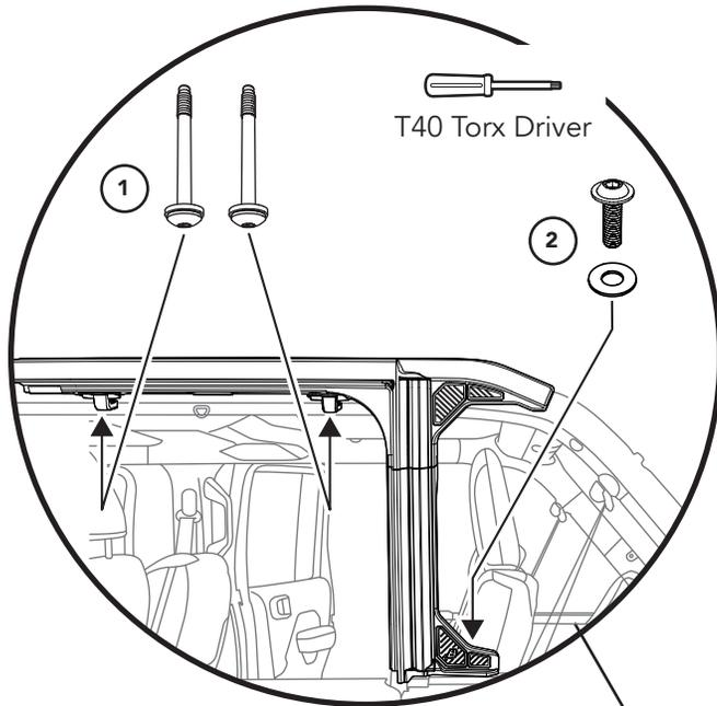
Attach the Rear Door Rail Assemblies to the Jeep. Place each Rear Door Rail Assembly onto the Jeep just behind the rear door.
