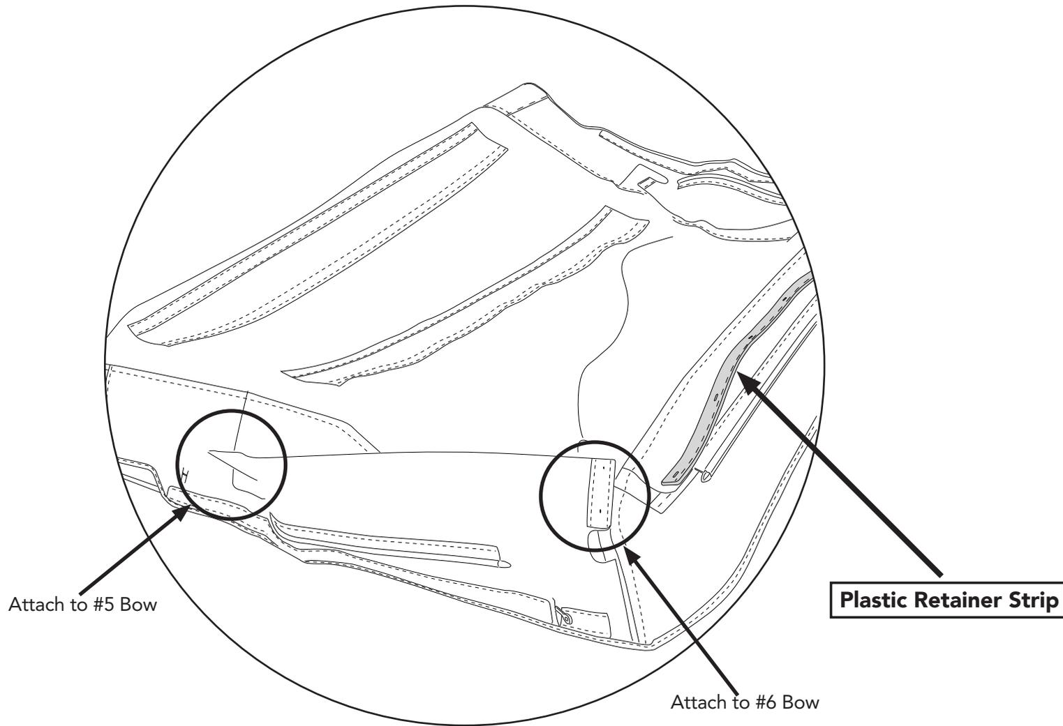
Lay out the Top Fabric Assembly with the inside facing up.
