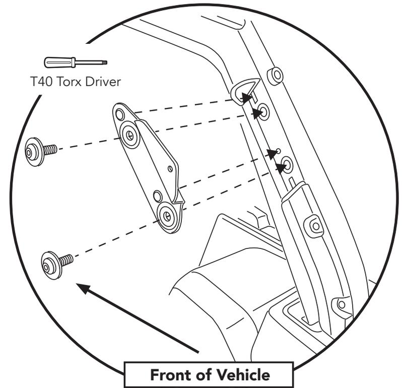
Attach the #6 Bow Support brackets to the sport bar down tubes. Place one pin in the small hole above the lower threaded insert in the sport bar and place the other pin in the slot above the upper threaded insert. Secure with two (2) M8 x 28 mm screws.
