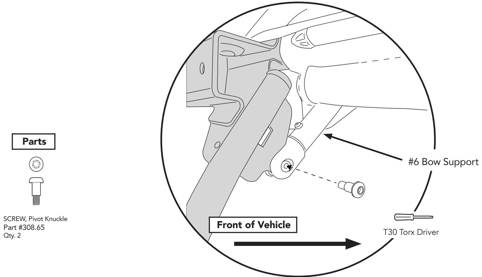
Pull the #6 bow down over the rear of the vehicle then attach the #6 Bow to the #6 Bow Support using one (1) Pivot Knuckle Screw per side.
