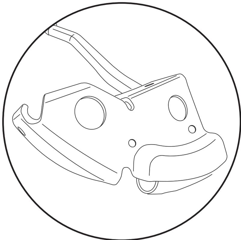
Insert a Grommet into the bracket at the end of the #6 Bow Assembly.
