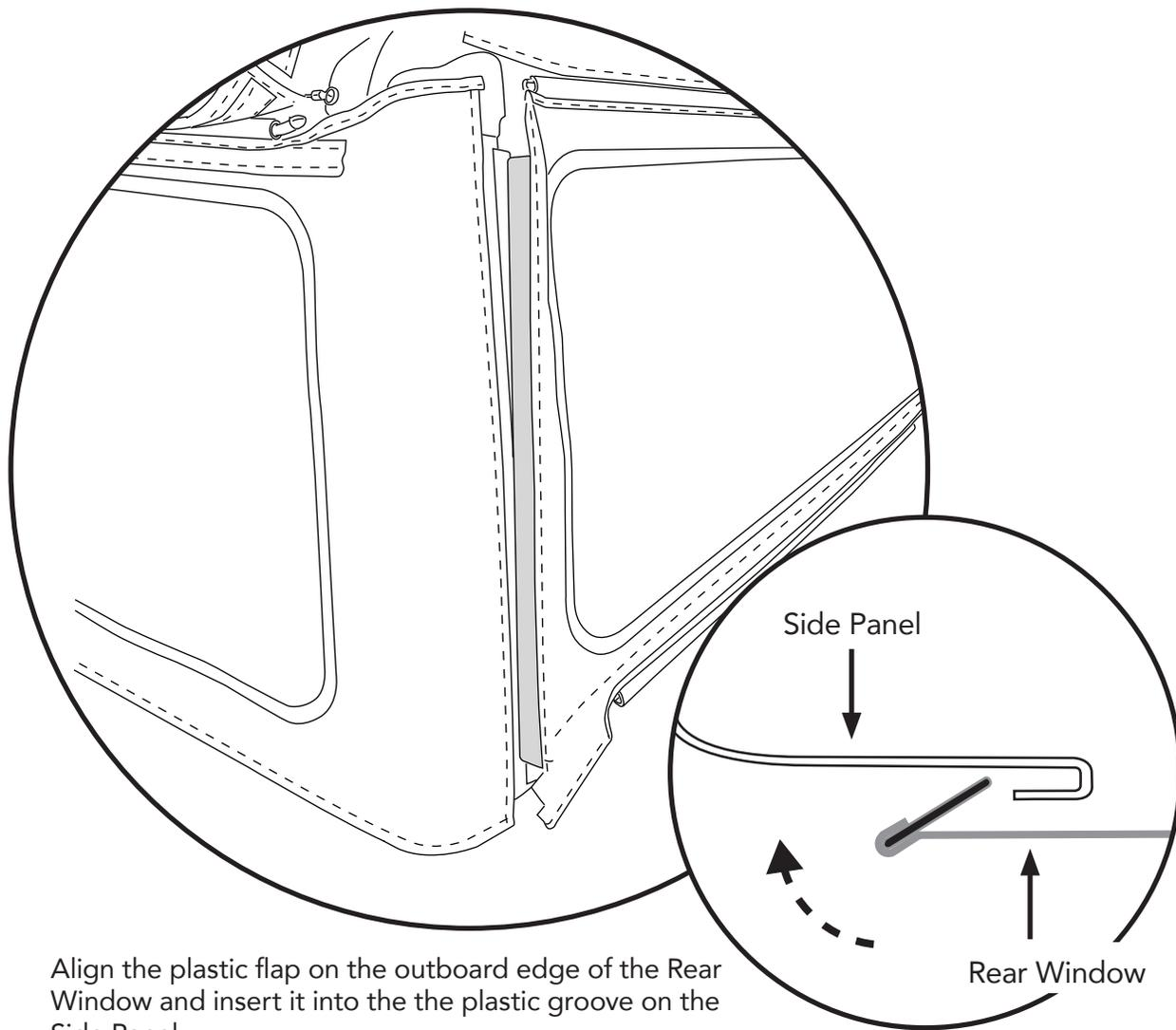
Align the plastic flap on the outboard edge of the Rear Window and insert it into the the plastic groove on the Side Panel.
