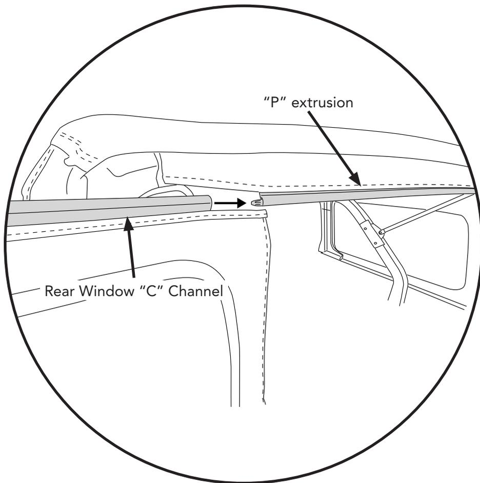
Slide the "C" channel from the top of the Rear Window onto the "P" extrusion located along the top of the rear window opening on the Top Fabric assembly.
