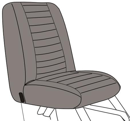
**Note:** On the driver's side seat, make sure that the fabric is tucked behind the seat adjustment lever and that the lever is clear to operate freely.
