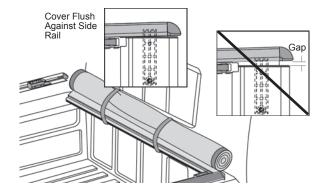
Locate the 2 side rails. Remove the protective tape on the bottom of each rail and place the rail on the bed on each side of the vehicle.
