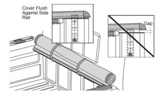
Once the rails are on the bed, align the front edge of each Side Rail, with the inside edge of the front bulkhead. Front of Bed
