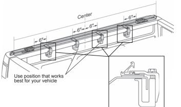
With the Tonneau Cover Assembly latched on both sides, push both Side Rails in so they are flush with the Front Rail. Center the front of the Frame from side to side on the vehicle.
