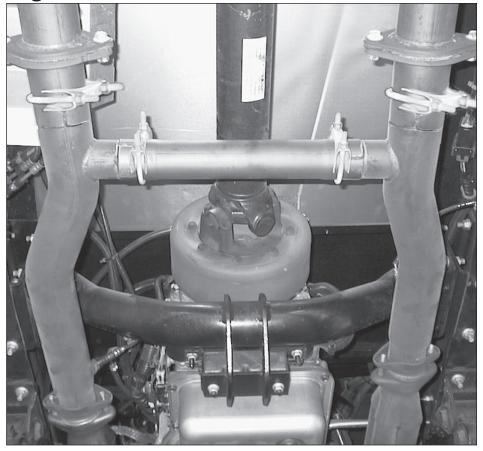
muffler inlet pipe onto the 2-bolt flange on the left-side intermediate pipe. Use (1) 2-bolt gasket, (2) 7/16-20 x 11/2" bolts, (2) crimplock nuts, and (4) 7/16 SAE washers for each flanged joint.
