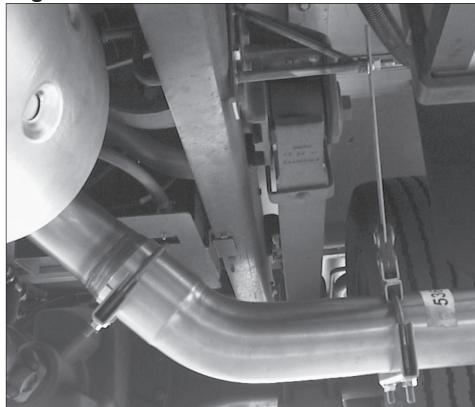
the extension. Also, be sure to leave at least 3.5-inches of straight on the tailpipe at the slip joint so it can be correctly inserted into the slip of the extension.
