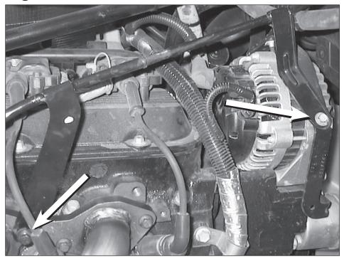
If the vehicle is equipped with inner front fender shields, remove them for improved access. If applicable, remove the two nuts securing the EGR tube to the rear of the rightside exhaust manifold.
