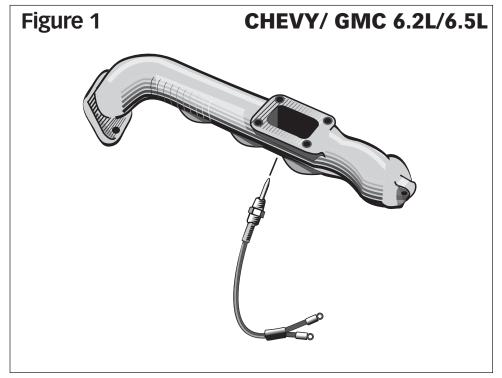
Mark a position on the exhaust manifold to locate the pyrometer sensor. Stuff a small shop towel or rag four to five inches into the exhaust manifold through the turbo mounting flange to prevent chips from entering the manifold while drilling and tapping.
