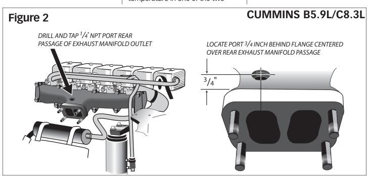
Tap the drilled hole with a ¼" NPT pipe tap. Check the thread depth as you tap by periodically removing the tap and screwing the sensor fitting into the tapped hole. The sensor should thread in three to three-and-a-half turns hand-tight.
