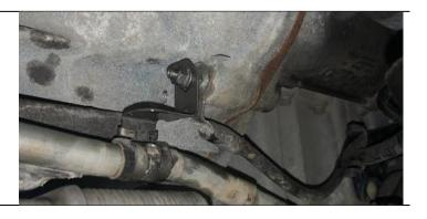
Reconnect the cooler tube retainer.
