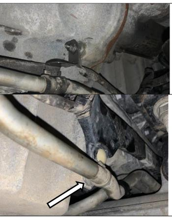
Unbolt the cooler line bracket holding the line to the front left of the engine oil pan.
