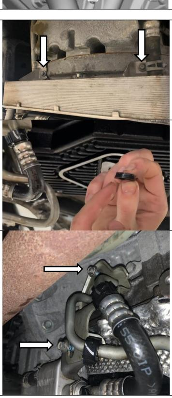
Reinstall the 4 stabilizer bar bracket nuts.
