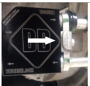
Reinstall both transmission cooler lines in to threaded end of the block, wiggle the lines and nut to start the threads. Tighten nuts 24 lb-ft.
