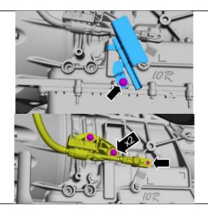
31. Remove fuel line bracket bolt.
