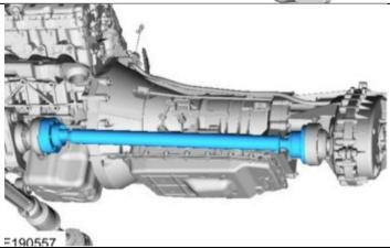
16. Remove the front driveshaft.
