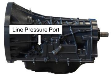
The line pressure service port plug thread is M10x1.00.
