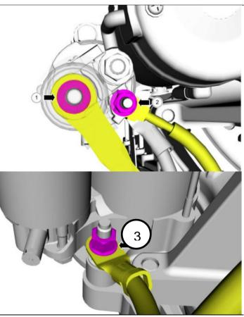
3. Remove the starter motor's three bolts and remove starter.
