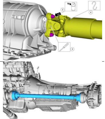
33. Install the rear driveshaft CV jointto-transfer case flange cup bolts and retaining straps.
