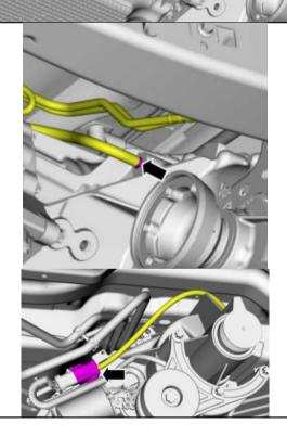
14. Install the selector lever cable bolts but keep the cable disconnected to the manual control lever.
