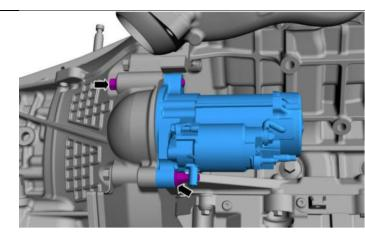
7. With the special tool (307-569), disconnect the transmission cooler outlet tube.
