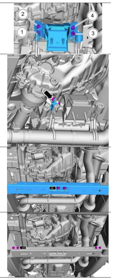
21. Install both LH and RH exhaust heat shield.
