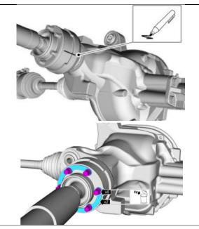
15. Index-mark the front driveshaft flange CV join-to-transfer case flange cup and then remove bolts and retaining straps.
