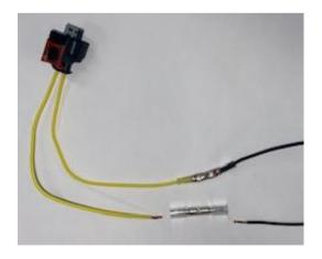
2. Connect new pigtail to injector
