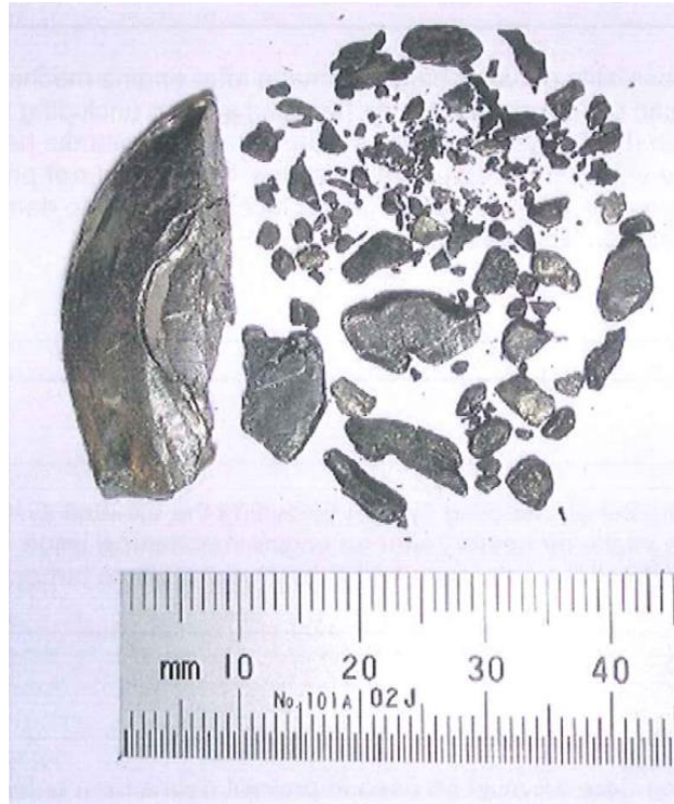
Figure 1 – Example of exhaust valve debris
