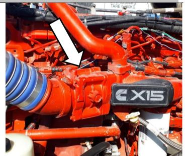
Locate the three screws securing the throttle body plate to the valve body.
