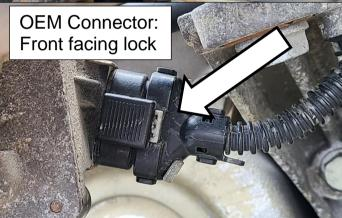
The connector lock on the BD harness is on the opposite side compared to the OEM connector.
