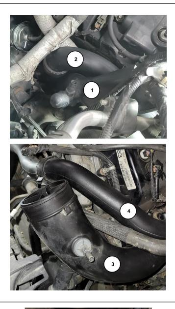
On the passenger side of the engine bay, Remove the nut securing the transmission cooler line support then slide support off of stud.
