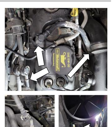
Connect the PCV pressure sensor electric connector, PCV tube quick connect couplings and install the PCV tube.
