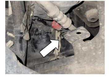
Disconnect the MAF sensor in the intake pipe.
