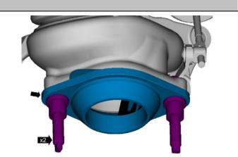
Install the new turbo gasket onto the turbo flange.
