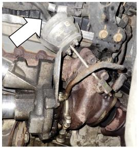
Remove the 2 turbocharger center housing bolts for the oil return tube.
