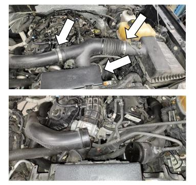
Disconnect the PCV pressure sensor electric connector, PCV tube quick connect couplings and remove the PCV tube.
