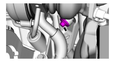
Install the 2 oil inlet/drain bolts. Tighten in the following stages:
