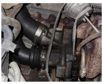
Disconnect the boost sensor and disconnect the pipe from the throttle valve and remove to allow for removal of the driver side turbocharger outlet pipe.
