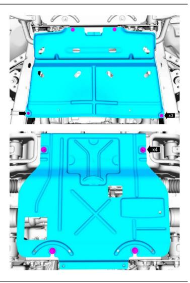
If equipped, remove the retainers and the transmission housing cover. Remove the bolts and the skid plate/splash shield.
