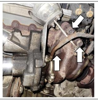
Remove the 2 remaining bolts holding the oil drain assembly.
