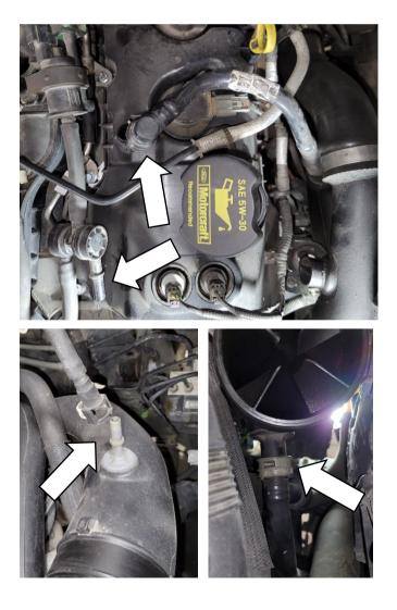
Loosen the clamps on the pipes which mount to the turbocharger and gently remove hose from the compressor cover.
