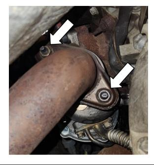
Remove the retaining clip in the coolant fitting on the top of the turbo and disconnect the coolant supply tube at the turbocharger.
