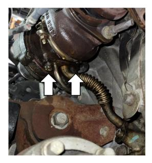
Install the oil return tube bolt at the cylinder block.
