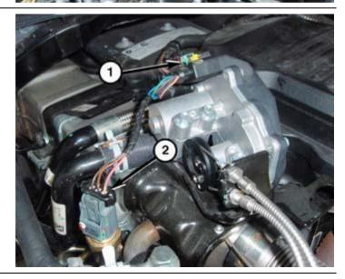
Disconnect the crankcase pressure sensor 2 wire harness connector (1)
