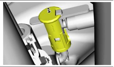
Connect the 4x fuel injector electrical connectors.
