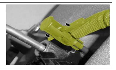
Push down on the center of the fuel injector return hose fittings to lock the fittings to the fuel injectors.
