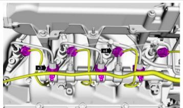
Position the RH and LH sound shields and install the 5 RH and 4 LH retainers.
