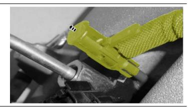
Remove and discard the fuel injector supply tubes.
