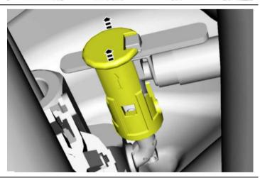
Pull up on the fuel injector return hose fittings to disconnect the fuel injector return hose fittings from the fuel injectors.
