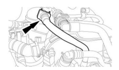
Install one end of a suitable hose onto the secondary fuel filter and the other end into a suitable container.
