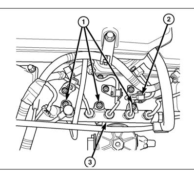
Position proper fuel line to proper injector on engine, tighten fittings hand tight at both ends of the line.
