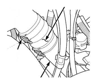
Remove the cables which are mounted to the intake heater grid.
