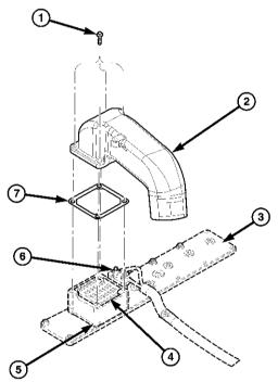
Connect rubber connector hose and intake tube to air intake housing. Tighten clamp bolts to 11 N.m. (100 in. lbs.)
