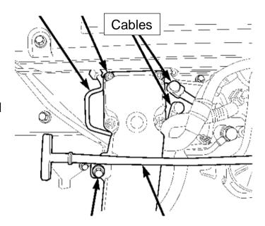
Remove wiring harness clips, engine oil dipstick tube bracket from air inlet connection and fuel filter housing, and the four housing mounting bolts (1).
