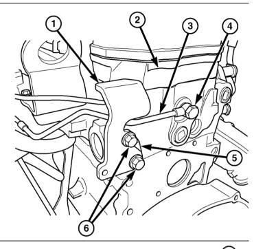
Remove necessary insulated fuel line support clamps (2) at intake manifold.
