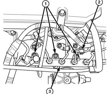
Place shop towels around fuel lines at fuel rail injectors. If possible, do not allow fuel to drip down the side of the engine.
