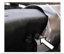
Align the catalytic converter with the manifold, and install the driver side transmission crossmember reinforcement bracket and bolts.
