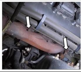
Ensure all gasket mating surfaces are clean and free of any debris.
