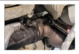
Install the air filter housing, filter, clear air hose and auxiliary air hose. Connect the catalytic converters to the resonator, torque spring nuts to **37 N-m (27 ft-lb)** Install the resonator supports, and torque bolts to **20 N-m (15 ft-lb)**. Install the engine cover and oil fill cap. Connect the battery. Start the engine and check for leaks.
