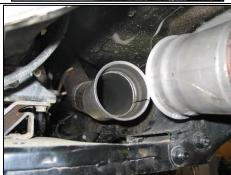
Install the brake valve between the two exhaust pipe adapters using the two supplied V-band clamps. Ensure the exhaust pipe adapters are in line with the brake valve to prevent possible leakage.
