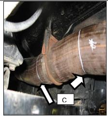
Cut out the marked pipe section using a reciprocating saw or cutting disk. Remove any burrs left on the edge of the pipe using a file or similar tool, then slide the pipe adapters onto the two cut ends of the pipe.
