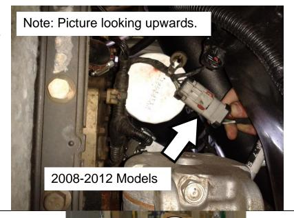
**IMPORTANT** Do not connect the harness to the EGR valve connector by mistake, it uses the same gray plug! Make sure the harness is connected to the VGT connector at the bottom of the motor.
