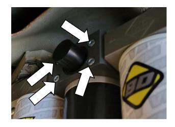
Install the 2x **1500313** fittings to both ends of the pump heads.
