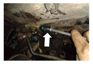
At the back of the engine (just behind the driver's side engine mount), disconnect the 1/2" feed line from the engine.
