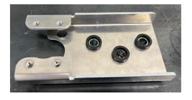
Mount the pump bracket to the frame bracket using the 3x **1900015** M8 bolts and 3x **1402609** M8 washers.
