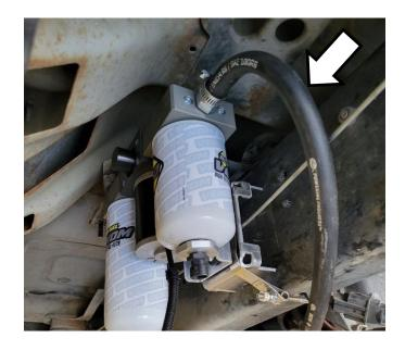
Install the supplied **1330157** 3/4" protective plastic loom over the hose for protection (not shown).
