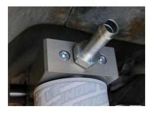
To connect the fuel supply line from the tank to the fuel pump, install the supplied 1/2" quick connect to hose adapter (1500394) onto the OE fuel line from the tank that previously connected to the HFCM.
