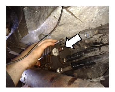
Install the fuel return line bypass tube into the two 3/8" quick connect fittings on the vehicle to reconnect the return line.
