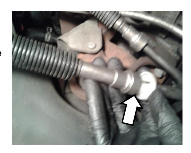
Now that the OE fuel feed line from the pump to the engine has been disconnected at both ends, it can be removed from the vehicle. Pop open the plastic bracket that supports the lines on the frame rail just behind the engine and remove the 1/2" feed line, it will not be reused. Refasten the bracket and leave the 3/8" return line in place.
