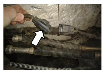
Undo the four quick connect fittings at the HFCM using a 3/8" and 1/2" quick connect release tool.
