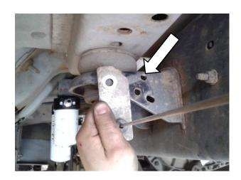
Insert the three vibration isolators in through the back side of the pump bracket.
