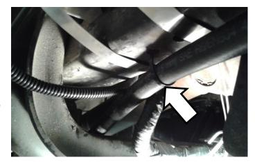
To connect the fuel pump outlet to the engine, connect a length of **1604054** 1/2" fuel hose to the fitting labeled OUT on the Venom pump or optional filter housing. Clamp the hose to the fitting using a **1452821** hose clamp. Route the hose over the frame rail behind the body mount.
