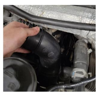
Gently remove the IAT sensor from the factory intercooler pipe by twisting CCW and lifting on the locking tab.
