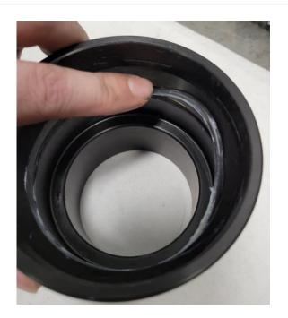
Slide the Throttle Valve Adapter into position on the engine and lock into place using the new locking clip supplied.
