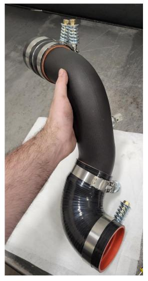
Install the assembled intercooler pipe into the engine bay. Slide the boot onto the intercooler outlet ensuring the rib becomes properly seated and flush against the intercooler as pictured
