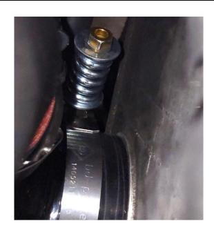
Slide the straight boot onto the Throttle Valve Adapter and align the components to ensure clearance on surrounding components.
