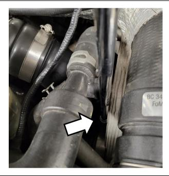
Remove the large metal E-Clip from the factory intercooler pipe at the throttle valve and pull pipe from throttle valve.
