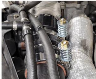
Once aligned, tighten all clamps until the tension springs are fully compressed.
