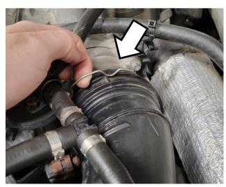
Loosen the clamps on the center silicone hump hose. Pull the plastic throttle valve adapter off of the factory throttle valve and separate from the lower pipe section.
