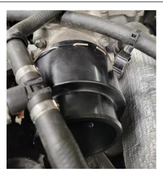
Insert IAT sensor into the adapter in the new intercooler pipe. Twist into position so that the sensor lock tab engages the raised locking feature.
