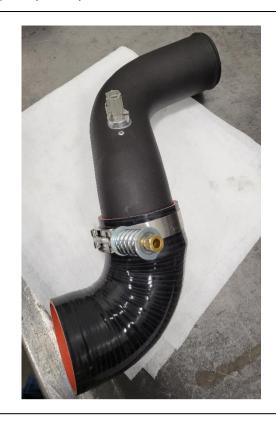
Slide the straight boot onto the intercooler pipe and place the clamps loosely into position on the pipe.
