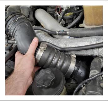
Pull on the pipe to disengage it from the ribbed feature on the intercooler. Remove the factory pipe assembly from the vehicle.
