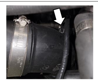
Loosen the lower intercooler pipe T-Bolt clamp.
