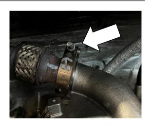
Use the supplied spring clamps (1500403), 3/8" diameter hose (1604053), and turbo coolant port block off plug (1462122) to block off the coolant port.
