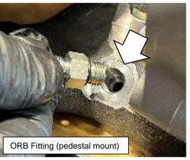
Connect the oil line to the two oil fittings, making sure that end of hose with a right angle connection is at top fitting.
