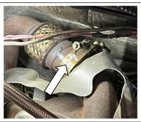
Loosen turbo feed pipe hose clamps.
