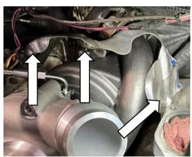
Mark position of the turbo outlet pipe (optional but highly recommended).
