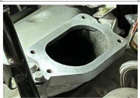
Install upper intake manifold.
