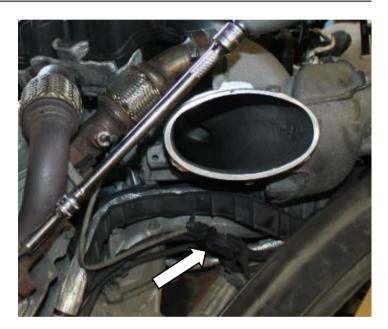
Connect CAC inlet hose and air filter inlet hose to lower manifold.
