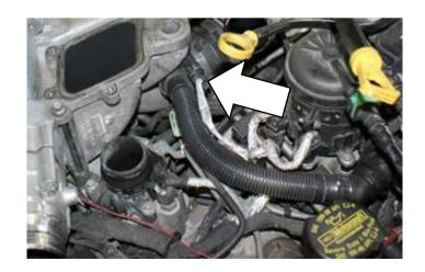
Reattach EGR bypass pipe and torque the 4 bolts to **10 Nm (89 in-lb)**.
