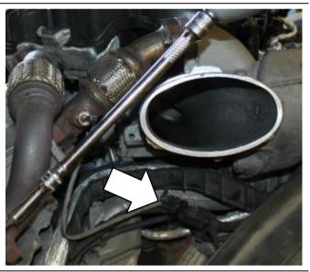
Remove 4 bolts and EGR bypass outlet pipe.
