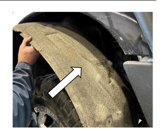
Remove upper downpipe elbow bracket bolt through RH fender well.
