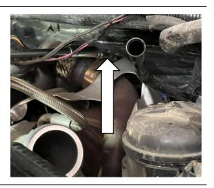
Remove heatshield. Three bolts hold heatshield to turbo as shown.
