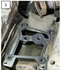
Ensure to pre-lube turbo oil inlet ports with ½ oz. of engine oil.
