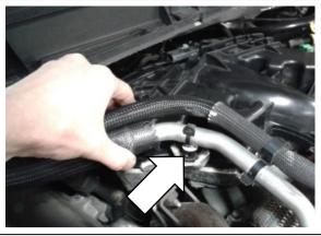
Disconnect turbo wastegate actuator tube on intake side as shown.
