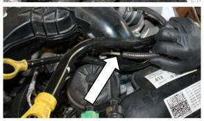
Remove wastegate actuator solenoid feed tube near the air filter intake inlet.
