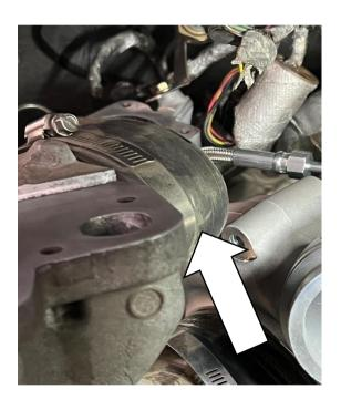
Reattach the crankcase vent tube by twisting it clockwise.
