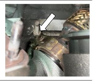
Seat upper downpipe to turbo, slide clamp into position, and torque to 15 Nm (133 lb-in).
