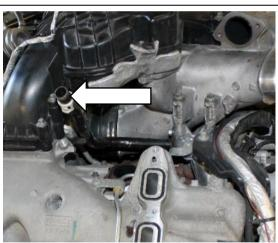
Mark position of turbo feed pipe clamps as shown (optional but recommended).
