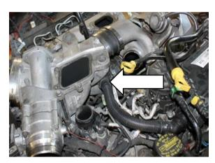
Release clip and disconnect Charge Air Cooler (CAC) outlet tube from Throttle Body (TB).
