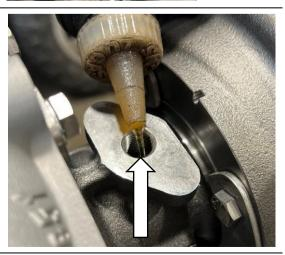
Add thin layer of thread sealant to NPT threads of **FT-420653**.
