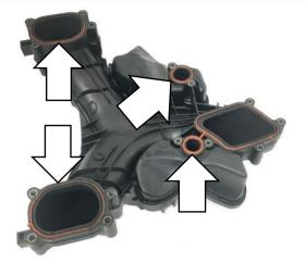
Before installing upper intake manifold, remember to remove rags or tape covering valve covers.
