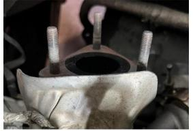
Replace feed pipe to manifold gaskets with the 2 provided **BC3Z-6N640-A**.
