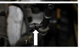
Remove transmission fluid level indicator tube bolt and engine oil level indicator tube bolt.
