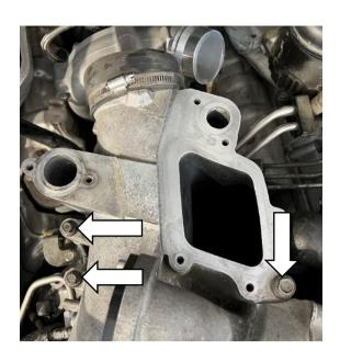
The Iron Horn does not utilize the top inlet boot. Use the provided **1405829** boot cap and remaining **FT-0427640** clamp to cover opening on the lower manifold.
