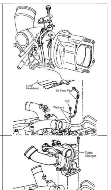
14. Remove the four turbocharger bolts and remove the turbocharger.
