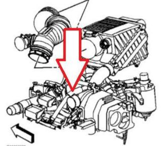
9. Disconnect both turbocharger coolant lines. Disconnect the PCV hose from the left rocker valve cover.
