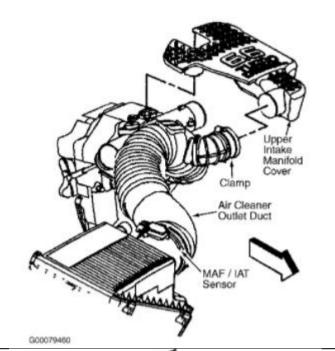
8. Disconnect the turbocharger air outlet CAC tube.
