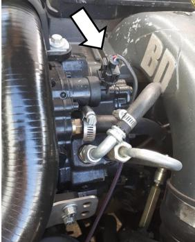
Mount controller in a safe area in the engine bay away from heat sources or belts and pulleys.
