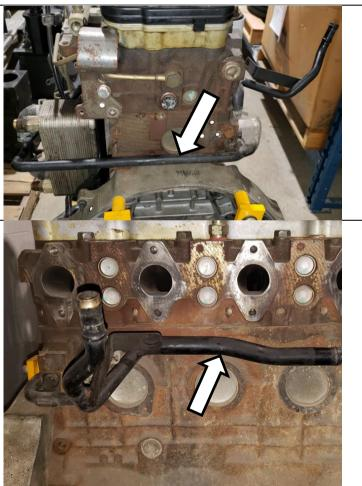
Finally remove the front section which connects to the water outlet fitting and then remove the water outlet fitting.
