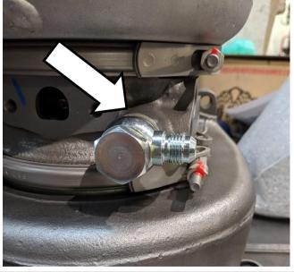
Install the speed sensor (1407043) into the turbocharger.
