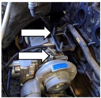
To help ease the installation of the manifold, it may be useful on 05-07 trucks to loosen the coolant tube and slightly shift out of the way.
