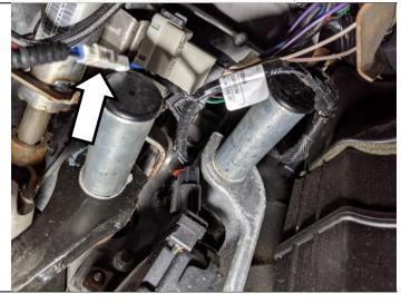
Route the RED and PINK wires from the toggle switch kit (1407038) from inside the cab to under the hood near the VGT control module.
