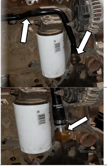
Mount the (1407034) coolant tube bracket (supplied from the Howler Install Kit) to the lower exhaust stud of the #6 cylinder reusing the OE M10 flange nut.
