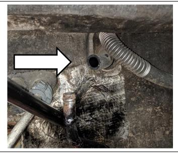
Cut the coolant hose as shown by the firewall. Do not discard the cut hose.
