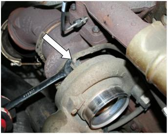
Remove the turbo oil feed from the turbo
