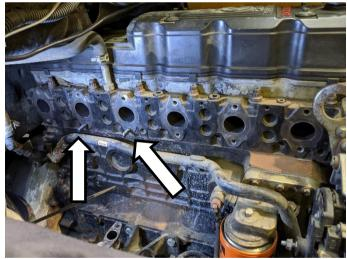
Remove the coolant port plug, towards the front of the engine on the passenger side.
