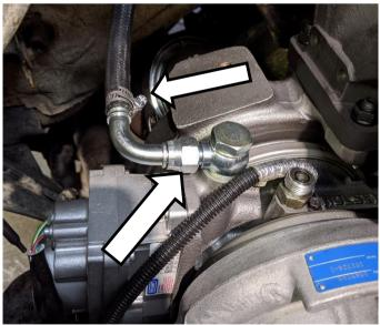
Install the two NPT plugs into the manifold if not using ports.
