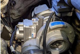
Secure the coolant line to the JIC fitting in the engine block installed earlier.
