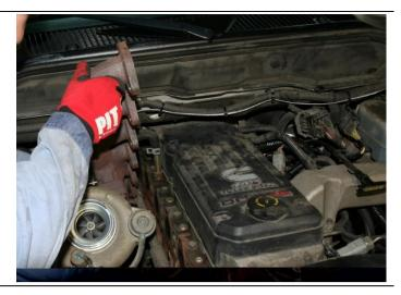
Special Note: Install Supplement Kit 1047137 which is for 2003-2005 automatic transmission models. This kit relocates the coolant pipes from the heater core/transmission cooler and water inlet connection from below the exhaust manifold to above. (Not required on trucks without a transmission oil cooler or when a coolant bypass kit has been installed)
