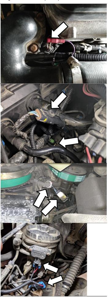
Choose the appropriate accelerator pedal position sensor adapter harness (1407130/31/32) for your model. Install this in line with the sensor.
