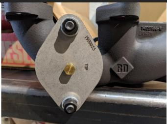
Install 2 of the longer studs in the engine as shown at the bottom of 2<sup>nd</sup> and 3<sup>rd</sup> port from the back of the motor.
