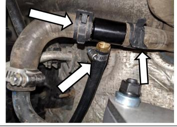
Install the JIC to Barb fitting. Secure the hose onto the fitting.
