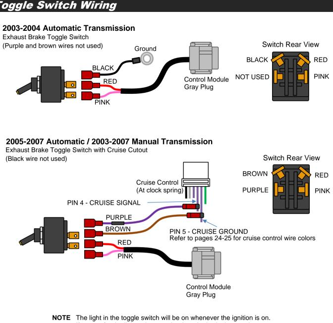
If you prefer the light to be on only when the brake is turned on, then reverse the RED and PINK wires at the toggle switch.
