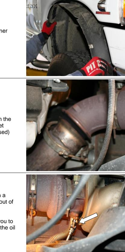
Remove the passenger side inner fender well with a 5/16" socket.
