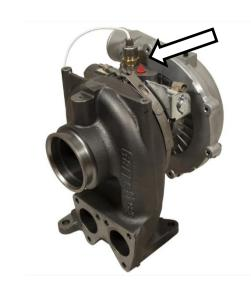
2. Install the oil return pipe using a new gasket.
