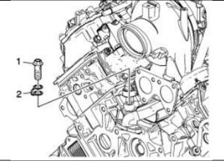
13. Install the turbocharger heat shield and bolts.
