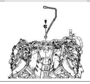
5. Install the turbocharger lower heat shield.
