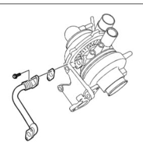
4. Install the oil feed pipe, washer, and bolt.
