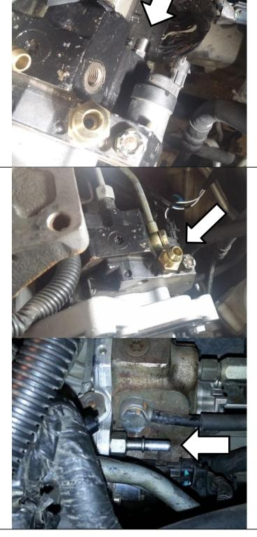
**5.9L Trucks:** Install supplied -8JIC swept fitting (PN 1502038) into the low-pressure fuel feed line using supplied gear clamp.
