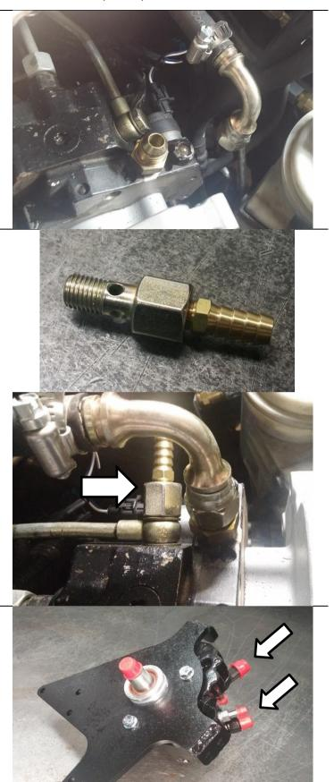
Mount pump and bracket to engine, using one (1) M8x25mm bolt and four (4) supplied M8x50mm bolts with four (4) flange nuts.
