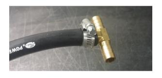
**Note** If using a fuel distribution block, connect the fuel hose to the supply port of the block instead of splicing into feed hose.
