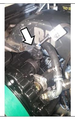
Double check to ensure all fittings are tight, then refill the truck with coolant and reconnect the batteries.
