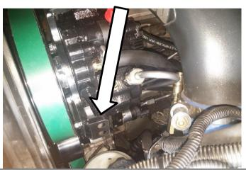
Install supplied upper radiator hose using the factory clamps.
