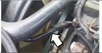
Using the T50 Torx bit, remove plug from lower driver's side rear of original cp3 pump in the truck.
