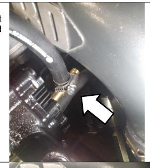
Trim the hose to desired length and attach to the ½" feed port on the second CP3 pump.
