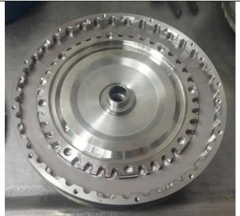
Reinstall the cover plate onto the torque converter.
