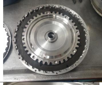
**Note:** Ensure the hub thrust bearing washers are not lost when the cover plate is removed.
