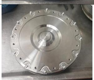
Once fully assembled, the end play of the torque converter should be verified, to ensure the stator spacing is correct. This can done by lifting the turbine using a end play tool, and measuring the play with a dial indicator <u>or</u> by using and end play gauge stand.
