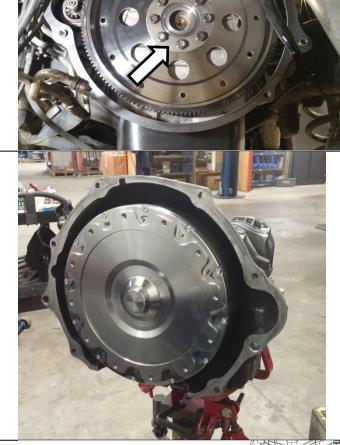
Install the transmission back into the truck.
