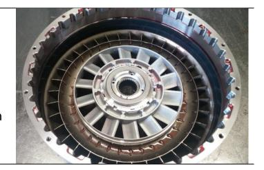
Assemble the turbine and piston into the impeller and install the clutch pack as outlined in the *Clutch Service* section of this manual.
