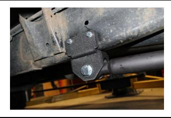
13. It is recommended to weld the frame mount bracket to the bottom of the frame.
