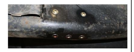
Mount both frame mount brackets to the frame using the 3/8"-16 serrated flange bolts.Use blue thread lock on all bolts and torque to 40 ft-lbs.
