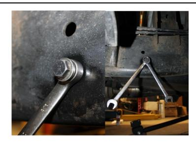
9. Remove the frame mount bracket from the traction bar and bolt onto the truck using the installed rivet nut. Ensure the bracket is located square to the frame and does not move during this process. Drill the four remaining bolt locations on each side using the bracket as a drill guide. Repeat steps 5 & 6, ensure drill locations are centered on the bracket holes. DO NOT interchange brackets between sides to mark locations.
