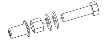
8. Place the rivet nut and assembly in the 17/32" hole. Tighten the 3/8" bolt while holding the rivet tool still. Torque to 23 ft-lbs.
