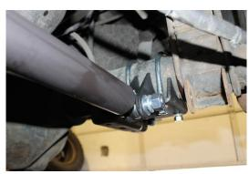
15. Torque the ¾"-16 jam nuts to 145 ft-lbs. Use a flat head screwdriver to centre the rod end during torqueing.
