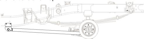
BD's traction bars are specifically designed to arc in the same path the axle travels during suspension movement. This makes for a smooth ride and the ability to tow without having to adjust the length of the bar. Other kits with longer rigid bars do not adhere to this design and will make the ride stiffer and cause suspension binding when the truck is loaded.
