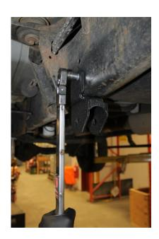
12. Loosen the axle brackets enough to rotate and insert the traction bar into the frame bracket. Fasten both sides in place using the 3/4"-16 bolts and washers (tighten to 223 ft-lbs).
