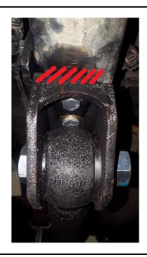
14. Use the ½" washers and tighten the ½"-13 U-bolts in a cross pattern to 95 ft-lbs. Ensure the U-bolts are square to the axle when installed.
