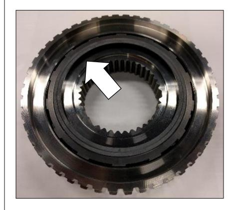
11. Flip the assembly over again and there should be a gap between the top face of internal gear and cage.
