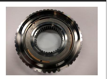
2. Remove snap ring and the retaining plate from the sprag and do not discard.
