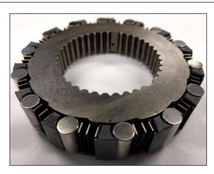
8. Lift and rotate the internal gear clockwise until the internal gear is sitting proud relative to rollers and cage.
