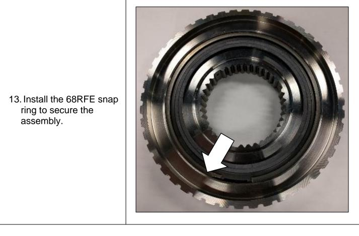
To ensure the assembly is correct, the internal sprag should only turn counter-clockwise and no rotation in the opposite direction.
