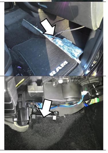
Unclip the plastic cover to expose the drivetrain control module. (4 clips)
