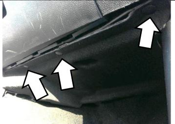
Disconnect the small wire for the under dash LED by pushing in on the tab to release it. Move this panel out of the way.
