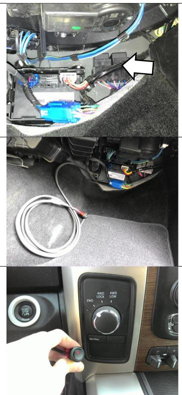
Using the stepper drill bit, create a hole to mount the switch. Use the small file to create a notch to locate the switch. The supplied decal may be used as a template.
