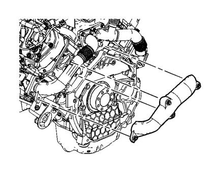
12. Using 12mm 12point socket wrench remove the driver side up pipe bolts.
