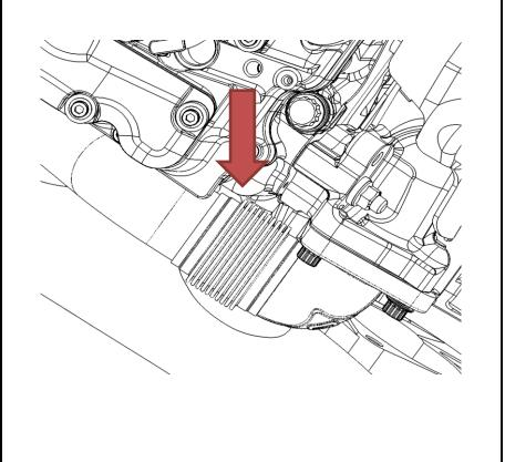
9. Tighten the exhaust up-pipe bolts in the sequence shown. Torque the bolts to 53 Nm (39 lbft)
