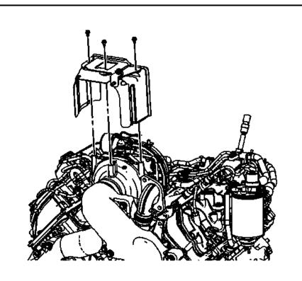
2. Loosen turbocharger exhaust down pipe turbocharger clamp nut (#1).
