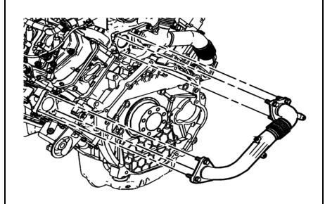
13. Using a plastic scrapper clean the feed port mating surface on the turbo and exhaust manifold.
