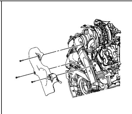
6. Using 12mm 12 point socket wrench remove the passenger side up pipe bolts.
