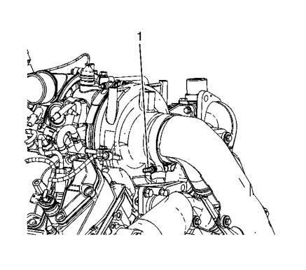
3. Remove turbocharger exhaust pipe to bracket bolt (#1). Remove the turbocharger exhaust pipe. If this is the OEM pipe you will discard as you will need an aftermarket one.
