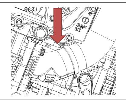
15. Tighten the BD-exhaust up pipe in the sequence shown. Torque the bolts to 53 Nm (39 lbft)
