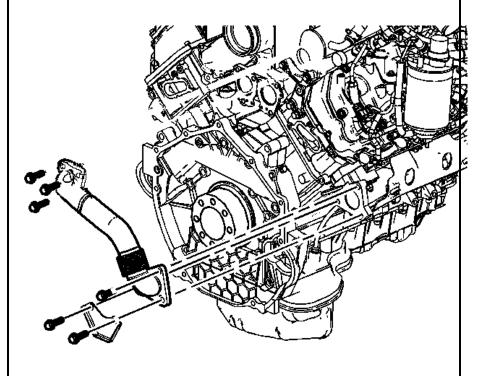
7. Clean up feed port mating surface on the turbo and exhaust manifold with plastic scraper.
