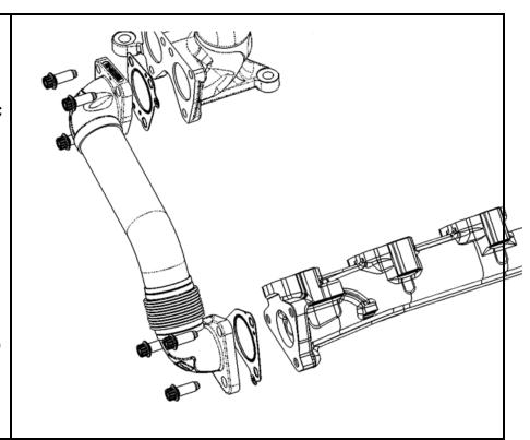
You must check for clearances at this critical point. Move the up-pipe to maximize this clearance.
