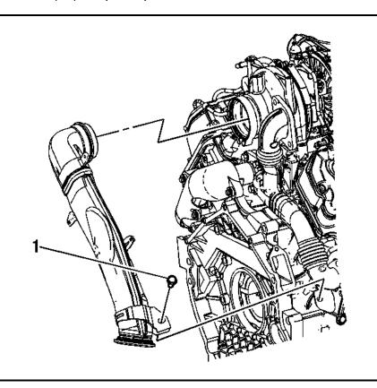
4. Through the wheelhouse opening, remove the transmission fluid fill tube to the bell housing.
