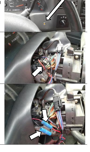
The shift lever wiring must be carefully secured to reduce chances of failure due to pinching or chafing.
