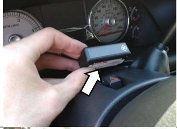
This location for the display is generally suggested as it does not block the gauges for most driving positions.
