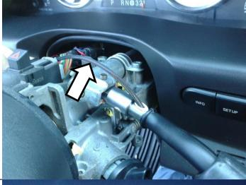
Move the shift lever through the gears and make sure the wire does not get pinched.
