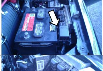
Remove the smallest of the three PCM connectors (towards the front of the vehicle) by releasing and rotating the gray lever lock.
