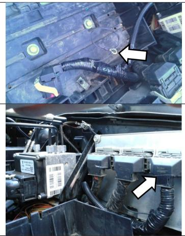
Reinstall the connector into the PCM.
