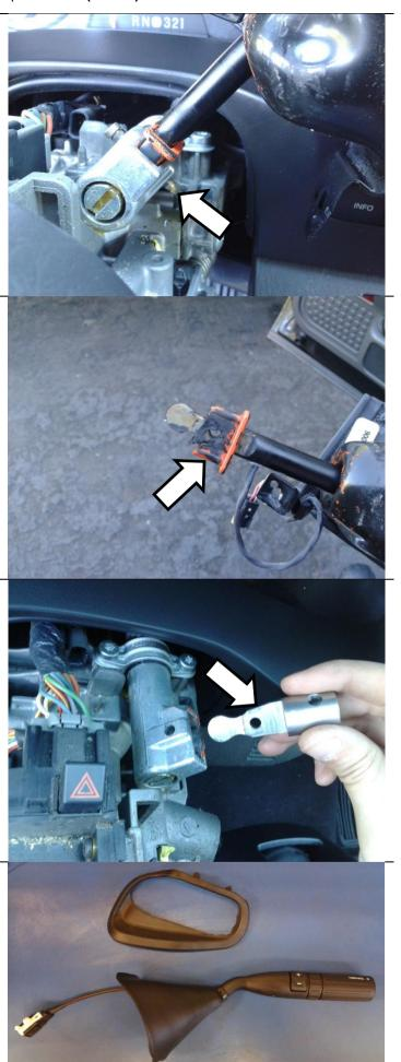
Install the new shift lever into the shift lever adapter. Slide the boot back on the shift lever to allow access to the mounting screw.
