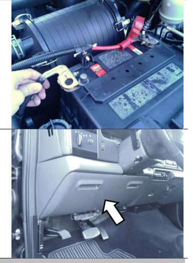
Remove the knee bolster below the steering column.
