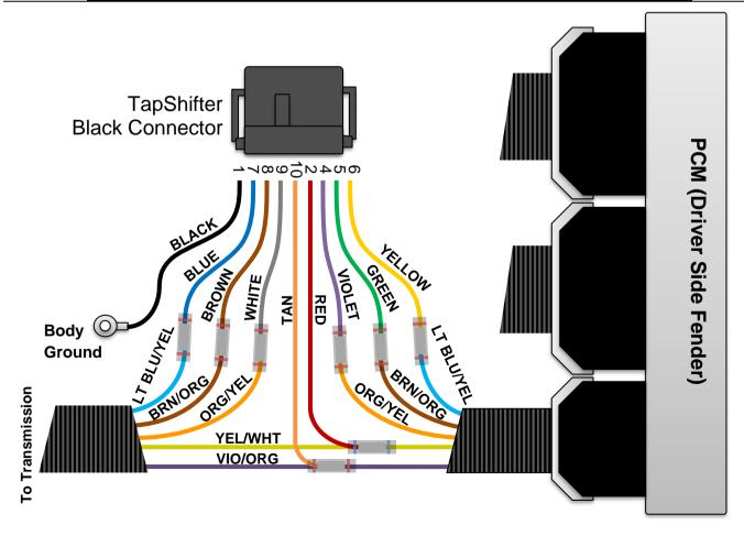
Incorrect electrical connections at the PCM are the number one cause of problems with this product. You may wish to test system operation before reinstalling the wire loom and taping up the wiring harness. The most common wire mixup is selecting the light blue/yellow OEM wire for the range sensor. This wire often fades to a gray color and is easy to mistake with another similar colored wire in the harness.
