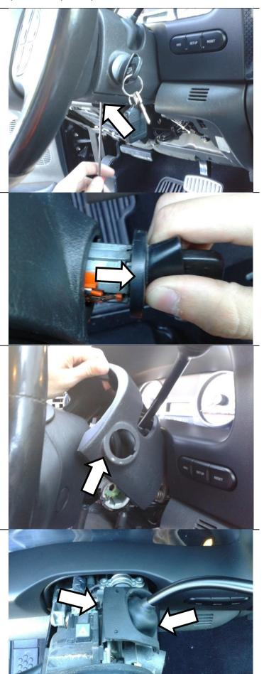
Using a punch and a hammer, drive the "press in pin" out of the shifter assembly. This will allow the shifter handle to be removed from the vehicle.
