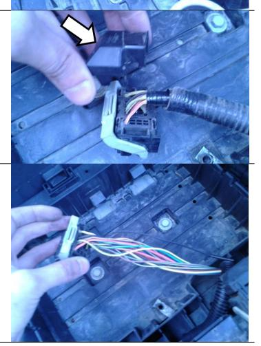
Remove the electrical tape from the wire loom to expose the wires. About six inches is sufficient to work with.
