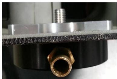
12. Now run your fuel line to the lift pump and cut to length. Secure the hose at both ends with the supplied gear hose clamps.
