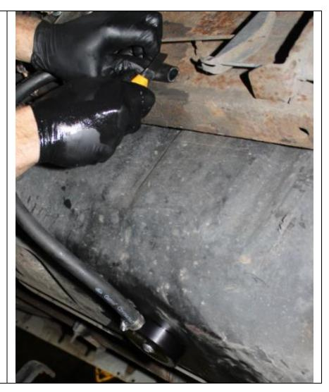
13. If desired, remove the old fuel supply line from the pickup and cap using the hose plug/clamp/fuel hose as shown. The larger of the two lines will be the supply, either 3/8" or 1/2"
