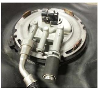
Note: If the sump leaks from the O-Ring, remove the sump and check the cut flange for burrs or cuts in the tank surface.
